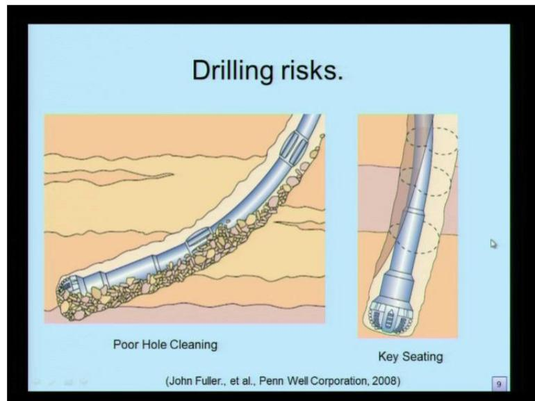
Further, it can also occur due to what we call a poor hole cleaning. You can see here, a residual deposit in the bore hole and this is not being cleaned or drifted properly and this can also result in what we call drill pipe sticking. Sometimes, this can also occur due to what is call key a seating. The key may not seat properly and due to that the drill pipe can also stick.
