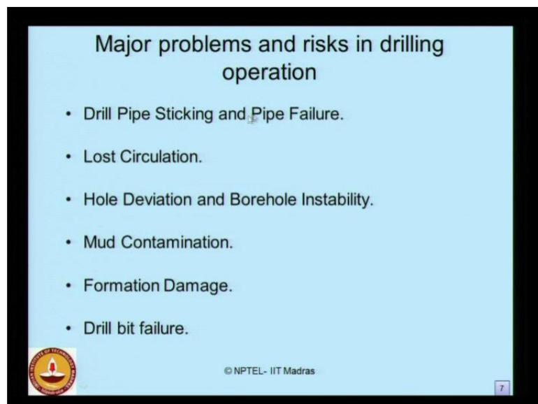
Let us ask a question, what are the major problems and risks that are seen during a drilling operation? There are many risks involved in a drilling operation. Very critical of them are mentioned here. For most, could be your drill pipe sticking and the pipe failure. The major problem can also occur due to lost circulation. It can be either from hole deviation and borehole instability. It can also occur from mud contamination. It can be
