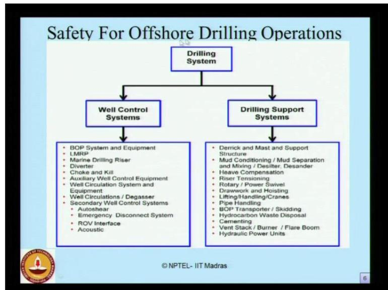
If we look at the safety measures related to offshore drilling operations. The safety measures can be categorized easily using this flow chart. The drilling systems essentially consist of two control mechanisms. One is what we call as well control systems; that are the control system available in the well. The other control system and support systems are available on the drilling area. Combined together is what we call as a drilling system.
