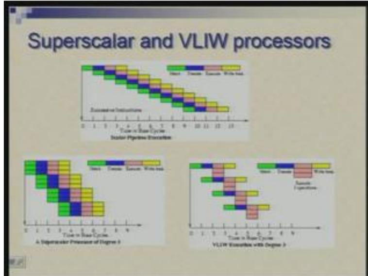
So, if you look at the timings of these two alternative architecture versus timing of a simple pipeline this is how it will look like. This top picture shows a four stage pipeline; let us say the four stages are: instruction fetch, decode, execute and write back. Then in ideal case you have instructions which are overlapping in this manner. So at any given time you have up to four instructions in flight.
