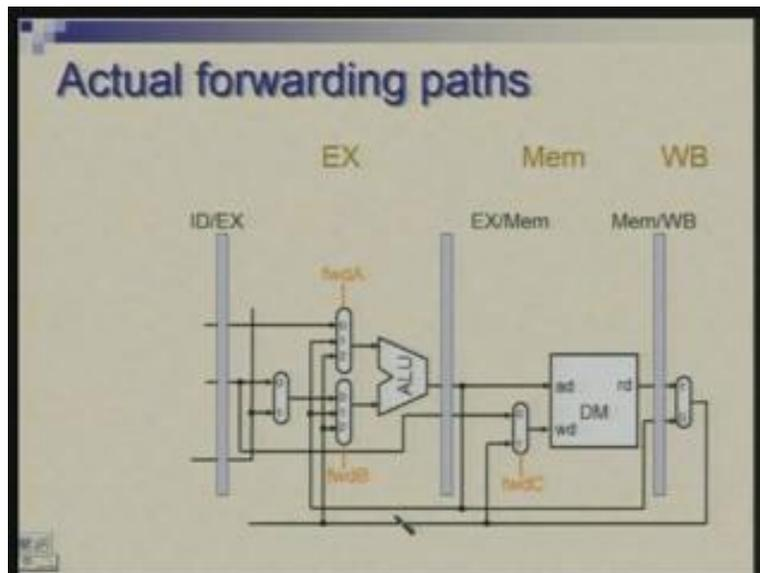
So, to improve things we had identified where we can have forwarding paths. So this diagram, for example, shows that you can have paths going from output of ALU through this inter stage register back to ALU or you could have output of the memory stage after this register and possibly after multiplexer going back to memory and also back to ALU.
