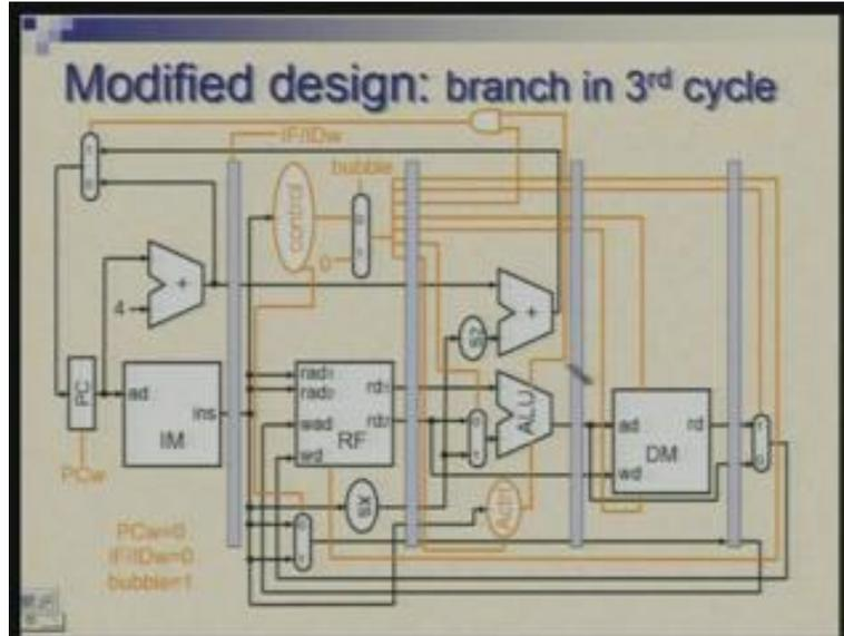
We are not making these pass through this register (Refer Slide Time: 7:42). The consequences of this are that the delay calculation which ultimately determines the clock period would undergo a change. Now you need to account for the multiplexer delay of this which we have ignored so far along with this adder and also with this ALU to consider the path delays.
