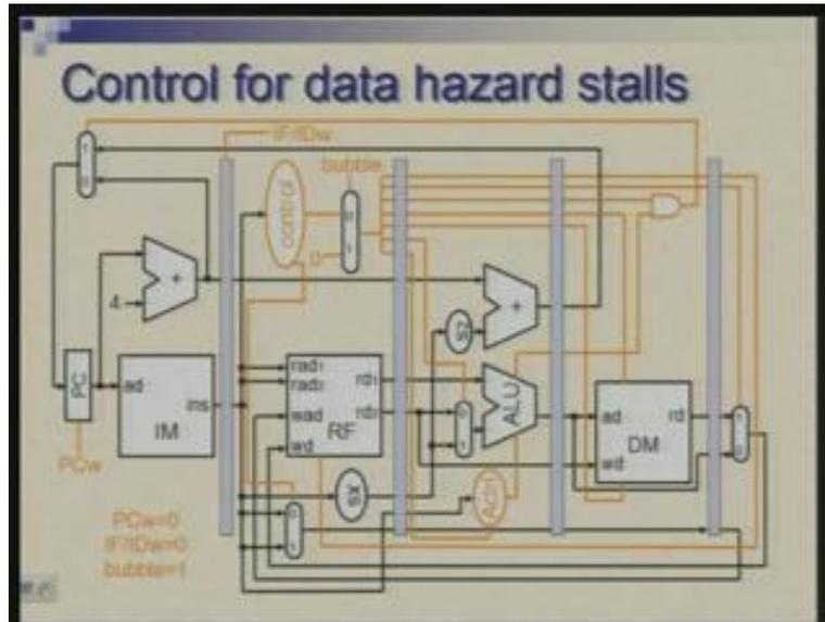
So now let us look at this design where you have datapath and control. It is same thing I might have re-rooted some wires just for the sake of clarity of the diagram. So now how do we introduce no operations and how do we prevent an instruction from moving forward.
