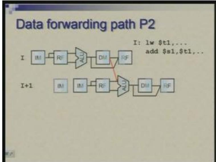
The only time this happens is that the earlier instruction is the load instruction because that is the only one which writes whether the result is ready after the fourth stage and the following instruction needs the result in the ALU stage. So we need to check this condition and we know how to introduce stall cycles; it is only the condition now we need to define freshly.
