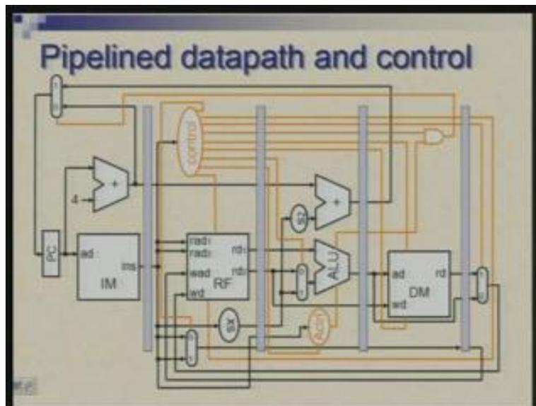
You have datapath and control which is much the same as single cycle control but again we make the control signal pass through the inter stage registers so that they are applicable at the right time.
