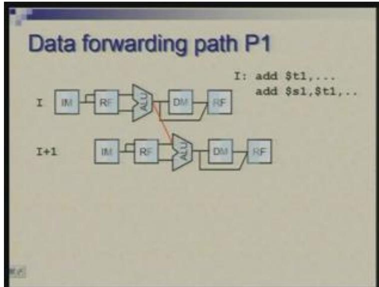
Yeah I think there is a situation where the delay introduced will be one cycle. The two dependent instructions are separated by one more instruction in between so in that case this match would occur (Refer Slide Time: 20:29) when the earlier instruction has reached DM stage and the one behind is in the RF stage. When the first instruction is in the ALU stage then it will not find any conflict there. So there could be situation where we introduce only one cycle.
