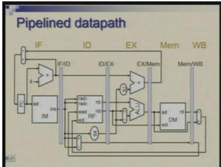
Here is the pipelined datapath which we have designed in the previous lectures and you would recollect that all we have done was taken single cycle datapath and introduced inter stage registers and after introducing controls this is how things looked.
