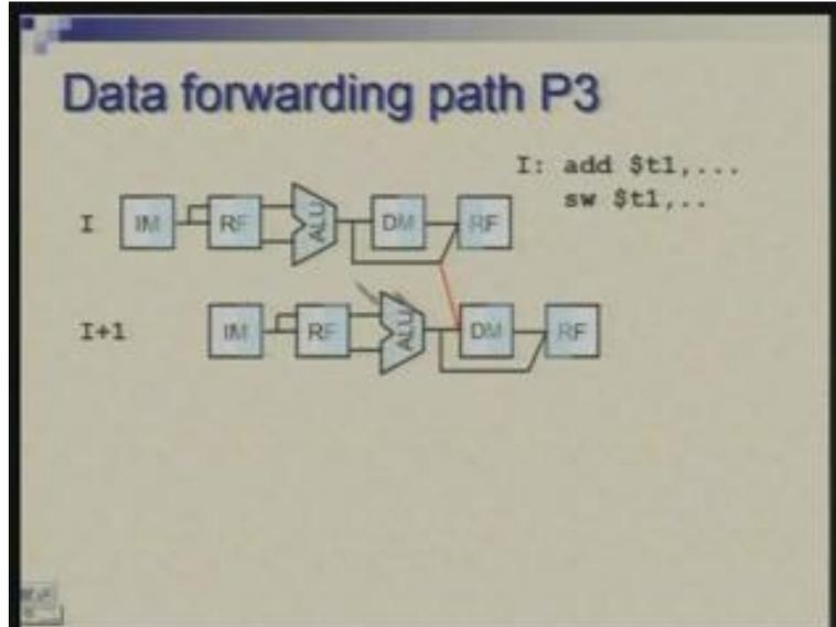
Therefore, now we do not pass directly from ALU to DM because that is no longer available that value would have moved to next stage so we will have to tap it after the DM stage and get it to input of the DM.
