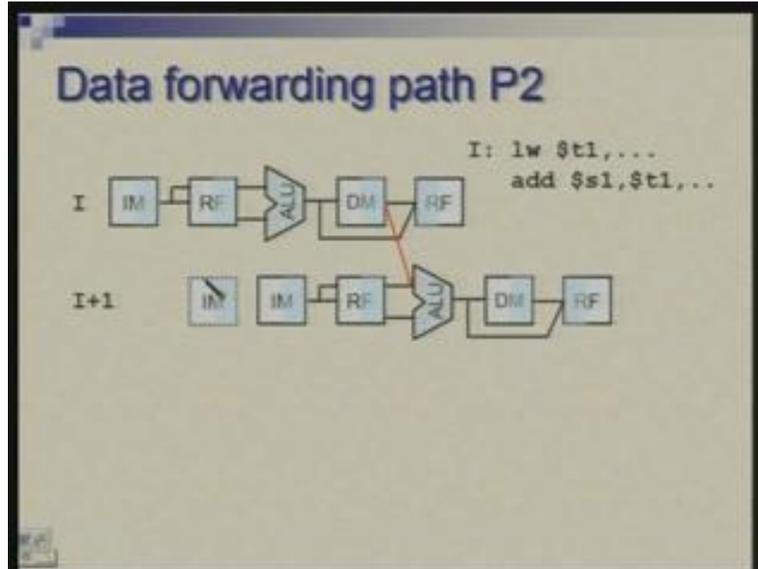
Another possibility is that a load instruction is followed by a dependent instruction like add. So in this case the data needs to be forwarded from DM state to ALU state and here you still need one cycle delay. Again this is not correct actually; we should show IM as a solid thing and RF as a dotted one here (Refer Slide Time: 22:03).
