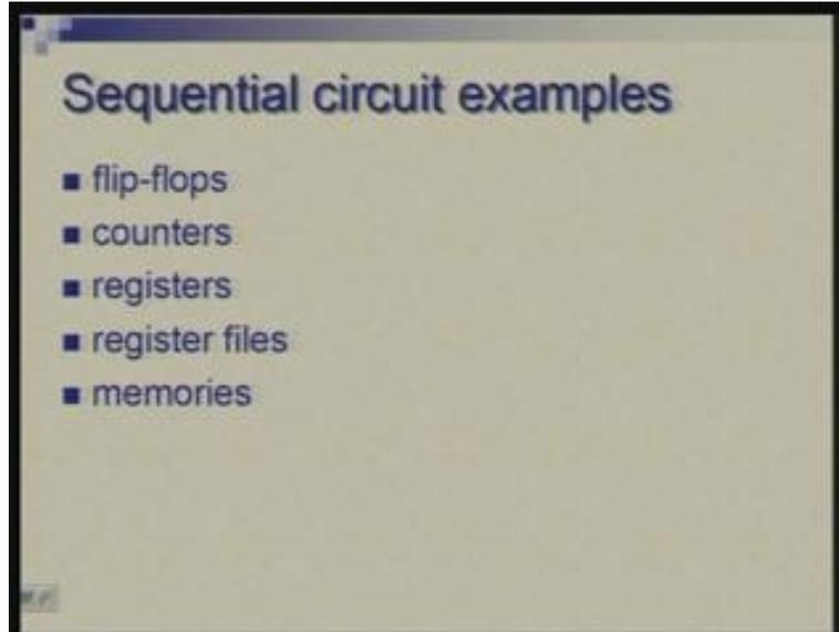
The most primitive ones are flip-flops which have one bit of memory; they can store a 0 or 1 depending upon what value they contain at any given instant of time depending upon the signals which occurred in the past.
