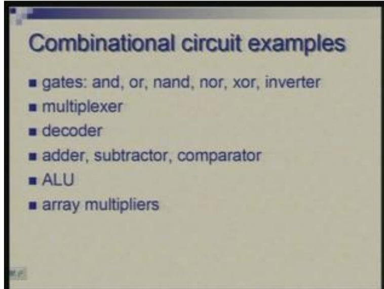
All gates are combinational circuits. If you take AND gate, depending upon what the input is it will almost instantly react to the inputs after some small delay. So, in ideal case we assume zero delay and say that the combinational circuits have output function of the current input. So various gates AND, OR, NAND, NOR, Exclusive OR, inverter and so on all these are combinational circuits.
