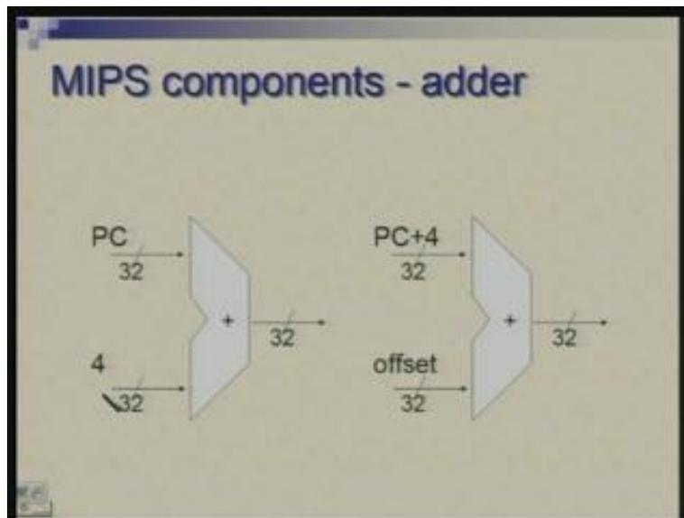
We will just put an adder where we need to add PC and 4. Similarly we are likely to have need for adding an offset to PC plus 4 for implementing branch instructions. For branch if the condition is true you are carrying out a relative branch. That means the offset which is specified by the instructions is added to the PC but we would have added 4 to PC by this time.
