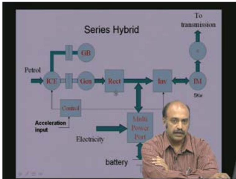
This schematic is called as series hybrid where the internal combustion engine is not directly coupled to the wheels; the internal combustion engine is coupled only to a generator which generates electrical energy and all the electrical energy is used for either charging up the battery or driving the induction motor which is the only thing which is connected to the wheels so it is called as series hybrid.
