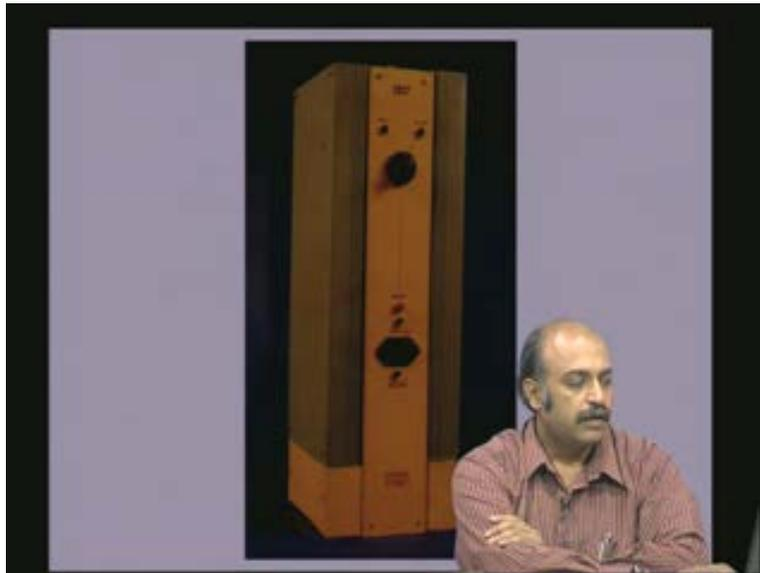
Now the output's electric power can be used for applications like powering various home loads or various office loads which are 230 volts. This is an inverter system where the input is photovoltaic just like your UPS system or input of the battery this is something similar with the input as solar photovoltaic cell and the output is 230 volts AC mains.
