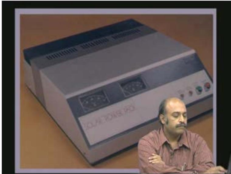
This is another useful application a standalone solar power pack where input is the solar PV and output is 230 volts which can be used to drive any home loads.
