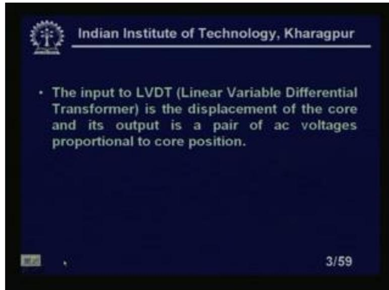
Now, the input to LVDT, which is linear variable differential transformer, is the displacement of the core. And its output is a pair of ac voltages proportional to the core position, as we know this is basic LVDT.
