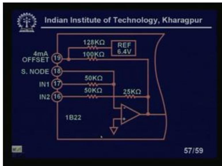
You can see here how the resistors networks are connected right? This is resistant networks in one B I mean this particular chip. What are internal networks? This are all inside the chip you can see where 6.4 volt reference voltage which can be generated by.
