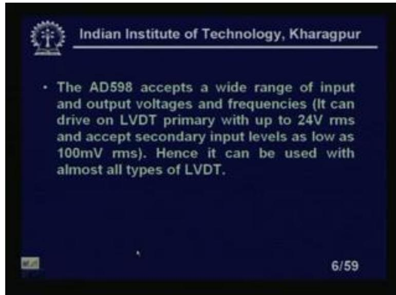
AD598 accepts a wide range of input and output voltages, these are all the features what it can and frequencies. It can drive on LVDT primary with up to 24 volt rms and accepts secondary input levels as low as hundred millivolt rms right. Hence, it can be used with almost all types of LVDT; that means, you please you see that LVDT and the primary can go up to 24 volt rms.
