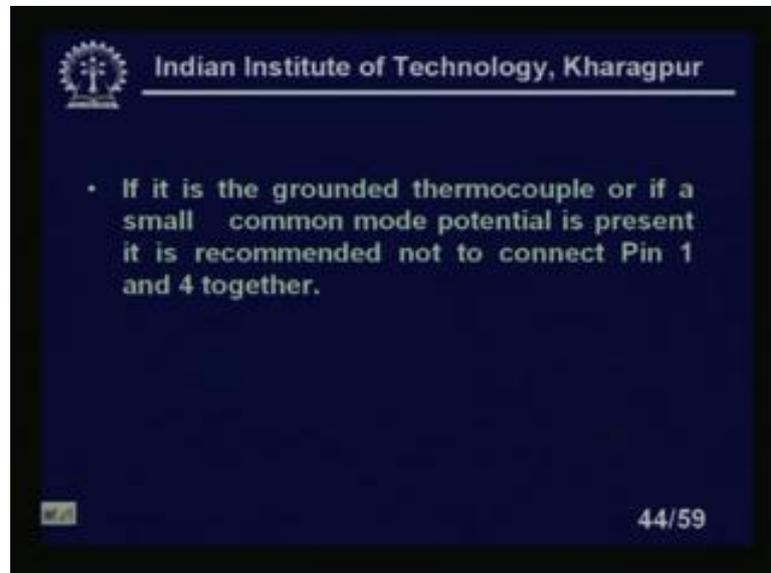
If it is the grounded thermocouple or if it is a small common mode potential is present it is recommended not to connect pin 1 and pin 4 together, right.
