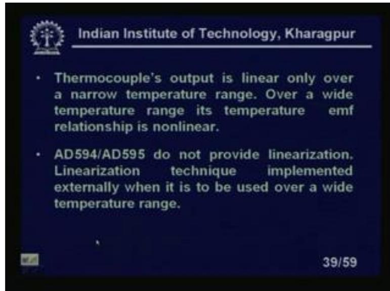
Thermocouple output is linear, only over a narrow temperature. That is you know thermocouple is non-linear devices over a short range only. I will get a linear characteristics, but however, it is a non-linear. So, you should take a wide range, if it is a if you can express at the polynomial equation, that I told you earlier also it looks like, if I take it is e naught sorry.
