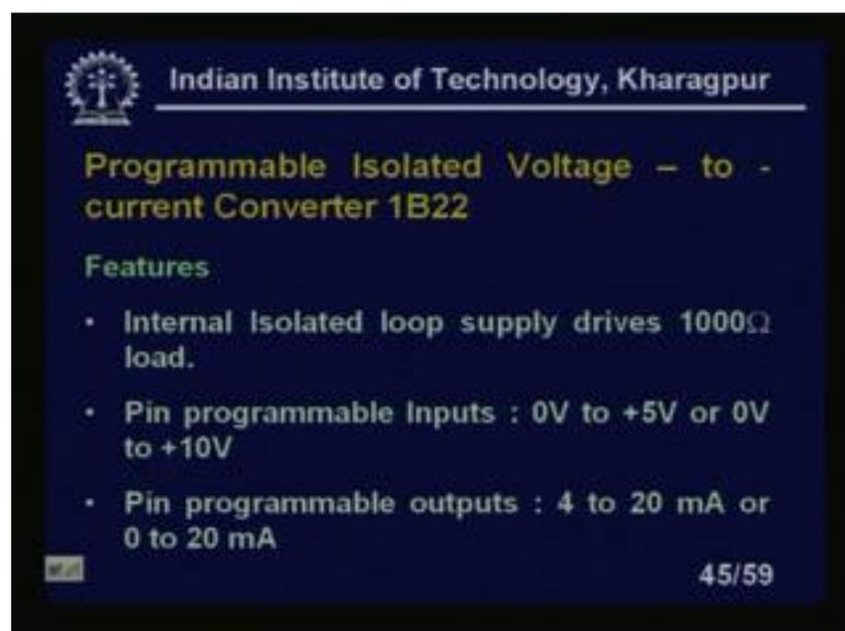
Now, last of this particular lessons we will discuss some programmable isolated voltage to current convertors 1B22. This is also many a places we need, because we cannot transmit current we cannot transmit voltage, we have to always transmit current. So, I
