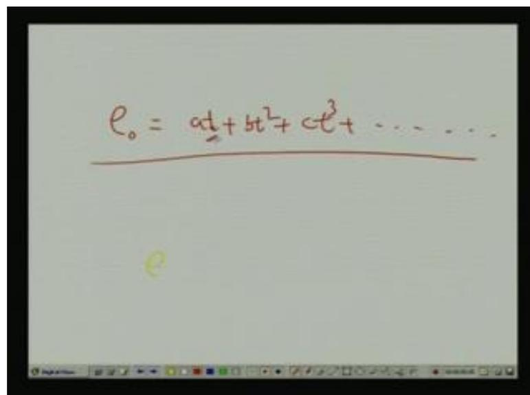
Output voltage  $e_0$  equal to  $at + bt^2 + ct^3$  right. So, it is the temperature created between the 2 junctions. So, it is the non-linear, you can see this one.
