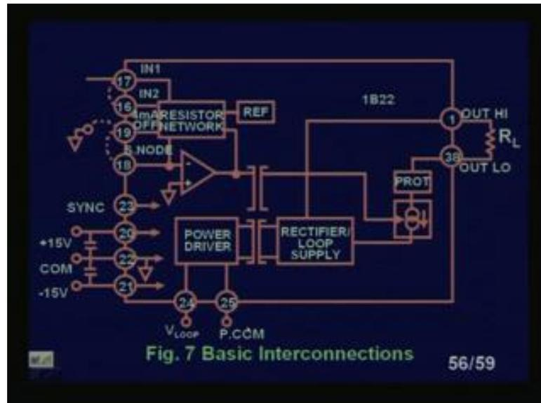
This is our functional diagrams you can see here how it works actually input 1 and input 2 these are resistor network 4 milliampere offset, we are using some capacitors here. So, we have a transformers we are showing like this one this are basic to transformer T 1, this is our T 2, this is a rectifier loop supply.
