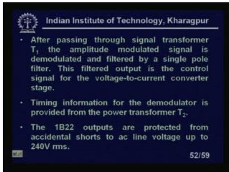
After passing to the signal transformer T 1 the amplitude modulated signal is demodulated and filtered by a single pole filter. That means, first order filter this filtered output is the control signal for the voltage to current convertor stage. Timing informations for the demodulator is provided from the power transformer T 2. The 1B22 outputs are protected from the accidental short circuit to ac line voltage up to 240 volt rms that is already I mean specified.
