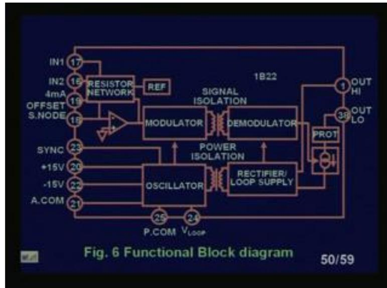
This is resistor network you see this is our basic block diagrams of our, this isolation you see the power isolation there is a signal isolation. So, all this isolation are there in this particular we have oscillators here this is our entire chip of this 1B22. This is an input input 1 and input 2, you can see which is coming the 4 milliamperere is to be keep I mean this one.
