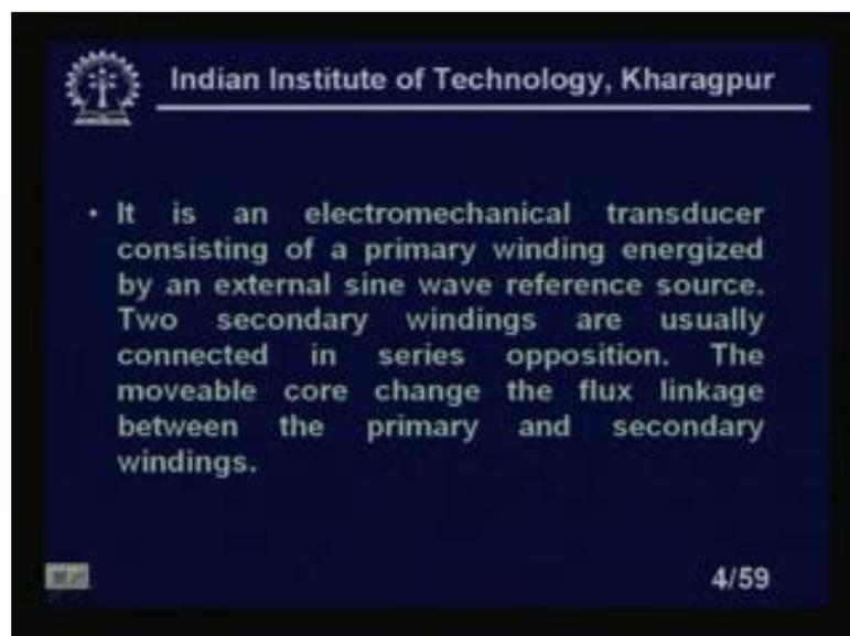
It is an electromechanical transducer consisting of a primary winding, energized by an external sine wave reference sources, external sine wave reference sources, please note always we need this source outside. And two secondary windings are usually, connected in the series opposition, this we have discussed in details. When we covered the LVDT
