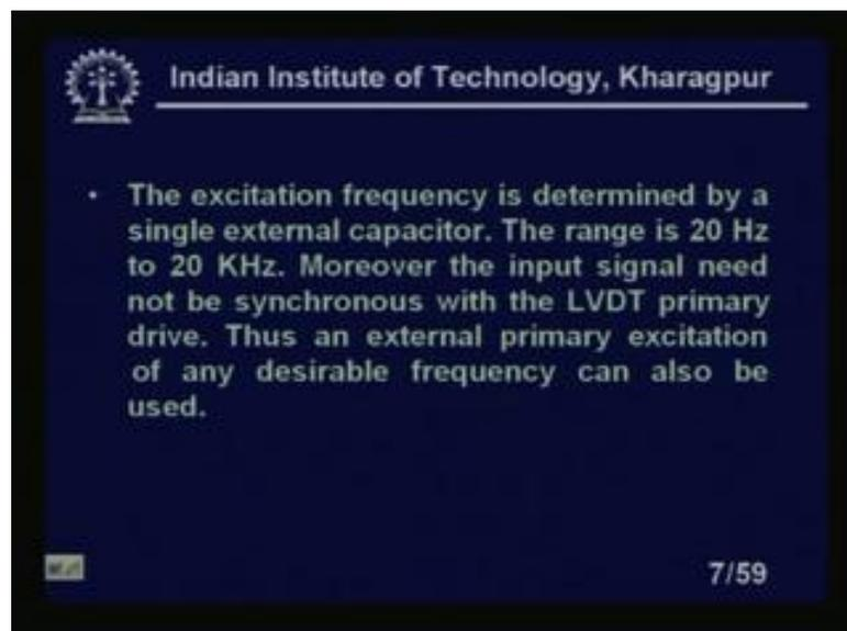
The excitation frequency is determined by a single external capacitor by using a single external. Which is outside the chip by excitation frequency of the LVDT can be I mean,
