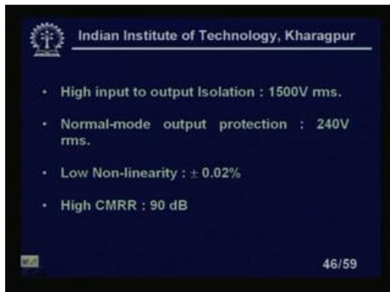
High input to output isolation high input to output isolation 1500 volt rms. So, it is a large isolation that is very much necessary to I mean to satisfy to protect my other instruments. Normal mode, output protection that is 240 volt rms. Low non-linearity it is plus minus 0.02 percent that is also greater advantage high CMRR it is 90 degree. So, common mode rejection ratio is quite high.
