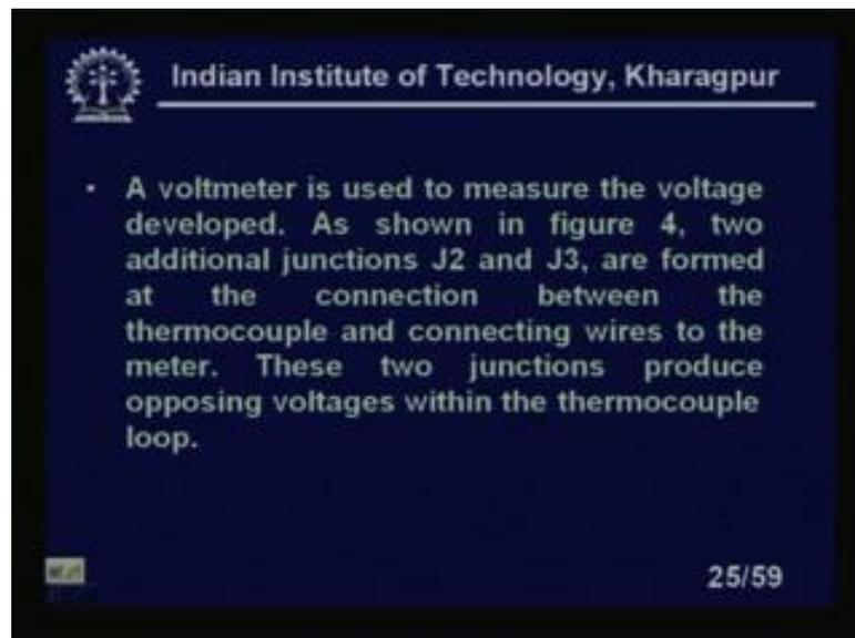
A voltmeter is used to measure the voltage developed as shown in the figure and 2 additional junction J 2 and J 3 are formed at the connection between the thermocouple connecting wires to the meter. Because that cold junction is not there in industry as I told. You excuse me these 2 junctions produce opposing voltage within the thermocouple loop right. So, one in most important things is that we have to this should be isothermal block I will show you in the next figure.
