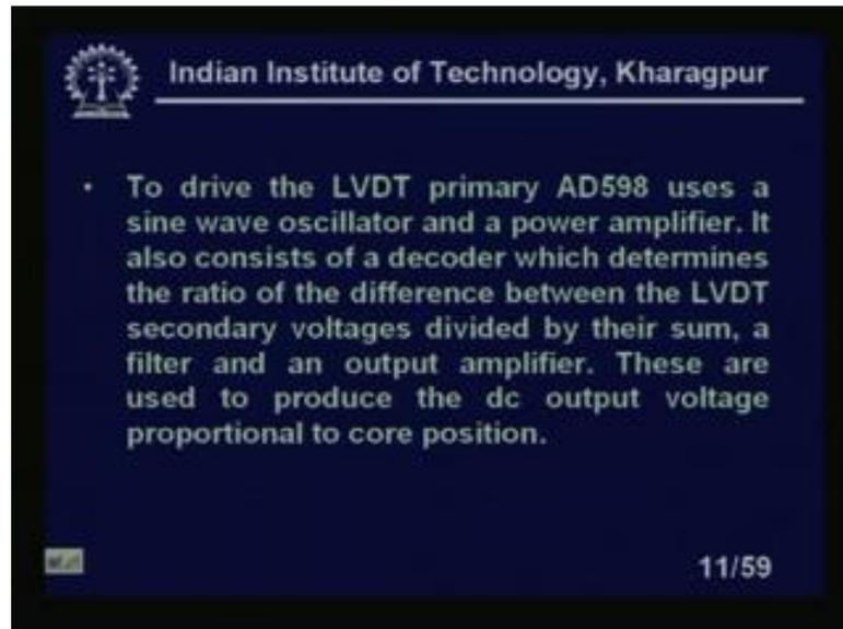
To drive the LVDT primary AD598 uses a sine wave oscillator and a power amplifier. It also consists of a decoder, which determines the ratio of the difference between the LVDT secondary voltage divided by their sum and a filter and an output amplifier. These are used to produce the dc output voltage proportional to the core position.
