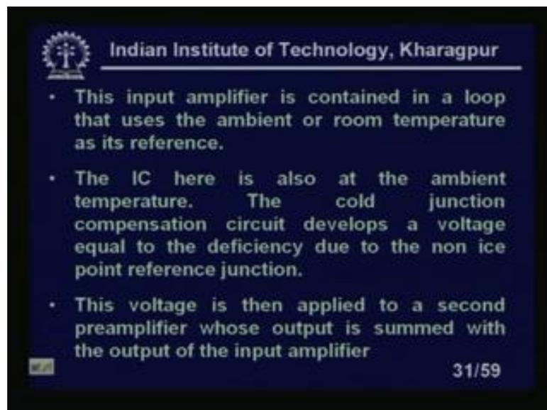
The input amplifier is contained in a loop that uses the ambient or room temperature as it is reference. The IC here is also at the ambient temperature and the cold junction compensations. Circuits develops a voltage equal to the deficiency due to the non ice point reference junction. The voltage is then applied to a second preamplifier, whose output is summed with the output of the input amplifier.
