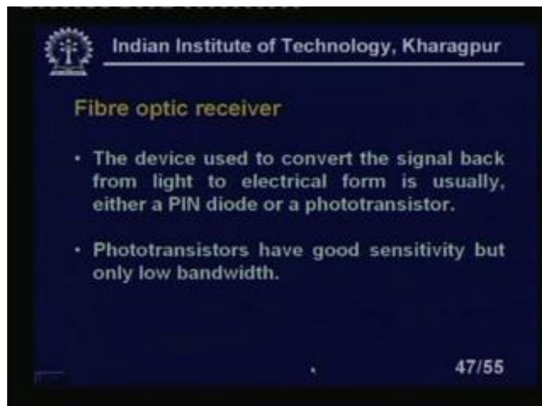
Fibre optic receivers device used to convert the signal back from light to the electrical form is usually either a PIN diode or a phototransistors right. Photo PIN diode is more popular use. Phototransistors have good sensitivity, but only low band width the bandwidth of the photo transistors is very small.
