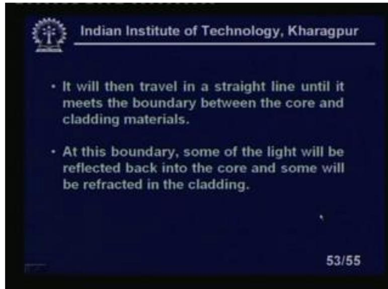
It will then travel in a straight line until it meets the boundary between the core and cladding materials. At this boundary some of the light will be reflected back into the core and some will be refracted in to the cladding, right.
