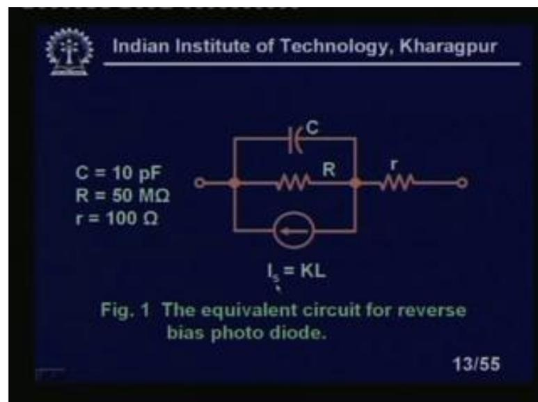
This is a equivalent circuit of a reverse bias photo diode. You see these, we have one capacitance, we have a current generator here  $C$  is equal to 10 pico farad  $P$  is I mean  $R$  is quite large 50 mega ohm and there is a small resistance  $r$  equal to only 100 ohm. So, is that saturation current is equal to  $K$  into  $L$ , what is  $K$ ?
