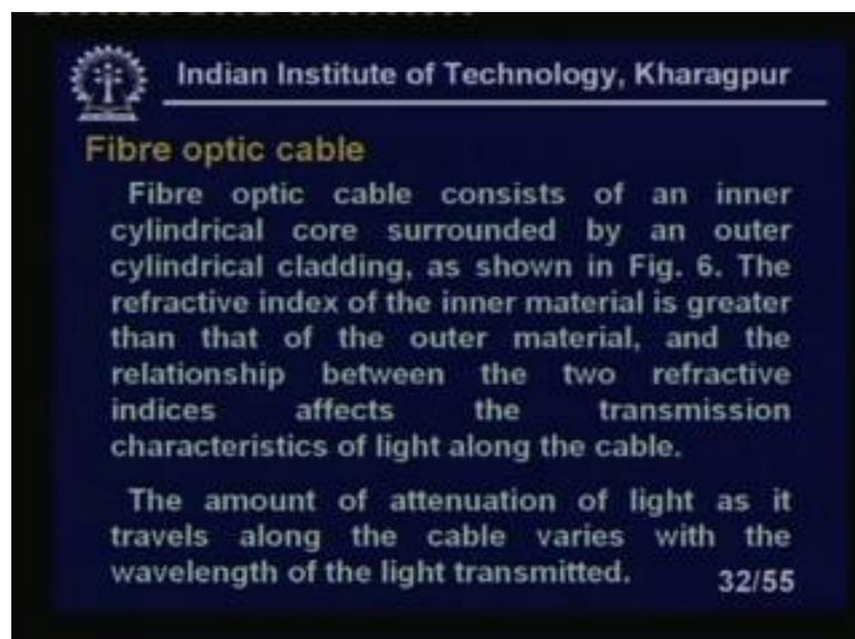
Fibre optic cable fibre optic cable consists, of an inner cylinder core surrounded by an outer cylindrical cladding as shown in figure 6. What is that figure 6? Let us look at a little far it went.
