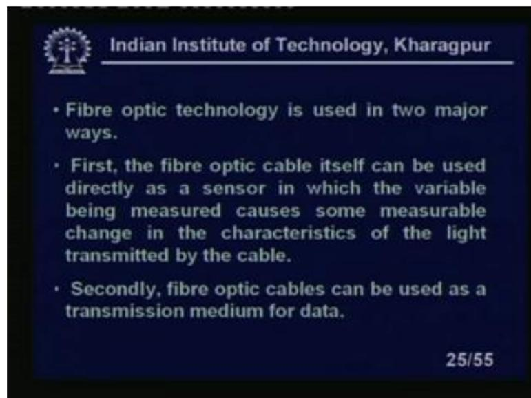
So, there is no ((Refer Time: 38:08)) as such. Fibre optic technology is used in 2 major ways, first the fibre optic cable itself can be used directly as a sensor, in which the variable being measured causes, some measurable change in the characteristics of the light transmitted by the cable. Secondly, the fibre optic cable can be used as a transmission medium for data.
