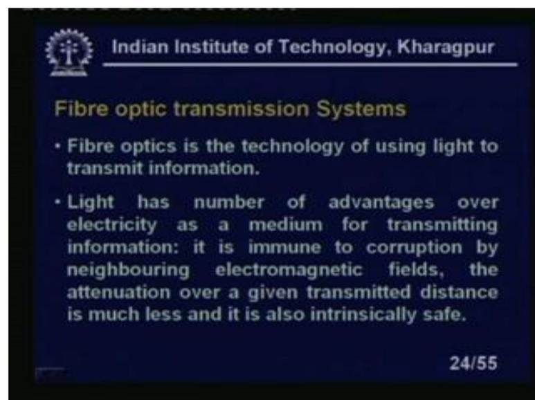
Fibre optics is the technology of using light to transmit information, light has a number of advantage over electricity, as a medium for transmitting information. It is immune to
