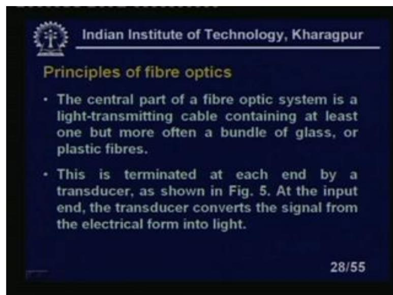
Principle of fibre optics; the central part of a fibre optic system is a light transmitting cable containing at least 1, but more often a bundle of glass or plastic fibres. This is terminated at each end by a transducer as shown in figure 5 at the input end. The transducer converts the signal from the electrical from into light, right.
