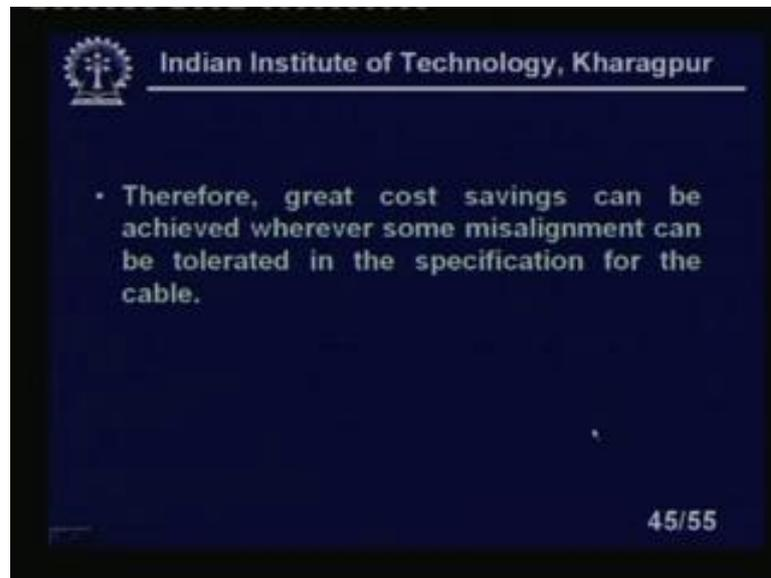
Therefore the great cost savings can be achieved wherever some misalignment can be tolerated. That is the reason multimode fibre is always preferred over the monomode fibre as little misalignment will not affect much.
