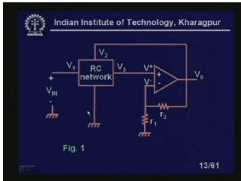
Because if you look at the circuit, you see that this is a positive feedback topology. RC networks in the positive feedback path, but if I keep the circuit as it is, circuit will
