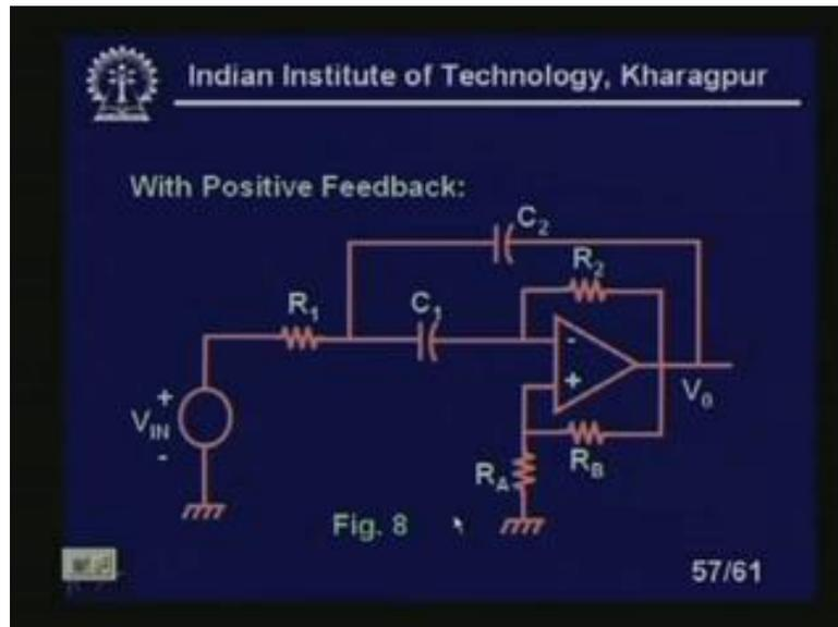
This is band pass circuits we have discussed, is not it? So, this is an enhanced negative feedback band, band pass circuit. That means negative feedback circuits with positive feedback. So, in band pass circuits, always it is desirable that the selectivity should be higher and higher. That is a good. Why? Quiet obvious, if I see there, here so that means what will happen? If I say, why I am telling?
