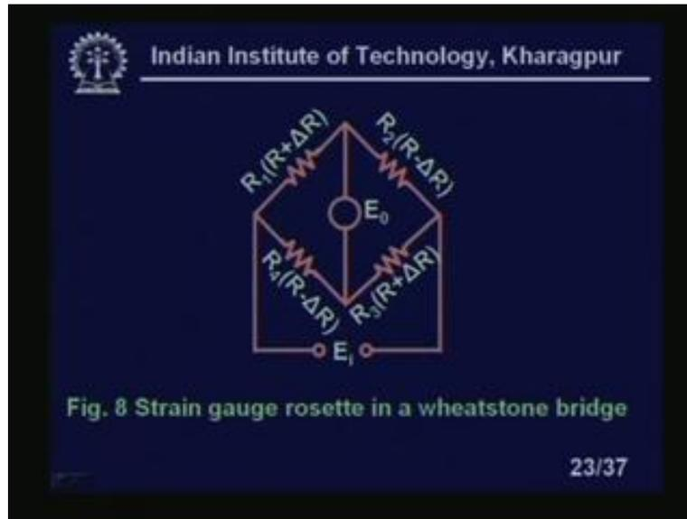
You see this is our strain gauge. R 1, R 3 which will basically sense the tangential stress, R 2 and R 4 which will sense the radial stress and it is compressive. So, it will be negative. So, resistance values are decreasing, here this is increasing. All are active gauges. So, strain gauge rosette in a Wheatstone bridge, so our output will be quite obviously ....
