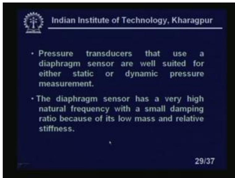
Pressure transducers that use a diaphragm sensors are well suited for either static or dynamic pressure measurement, quite obviously. The diaphragm sensor has a very high natural frequency with a small damping ratio, because of its low mass and relative stiffness.
