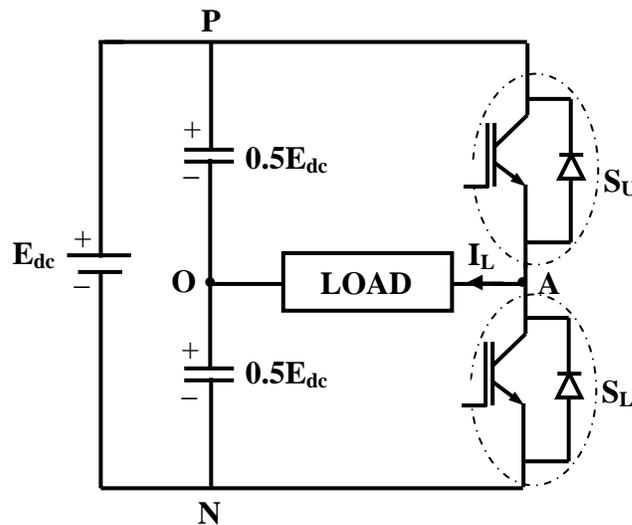
**Fig. 36.2: 1-phase half bridge VSI for CCPWM control**
