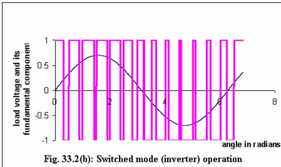
**Fig. 33.2(b): Switched mode (inverter) operation**
