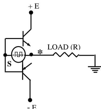
**Fig. 33.1 (b): A push-pull switched mode circuit**
