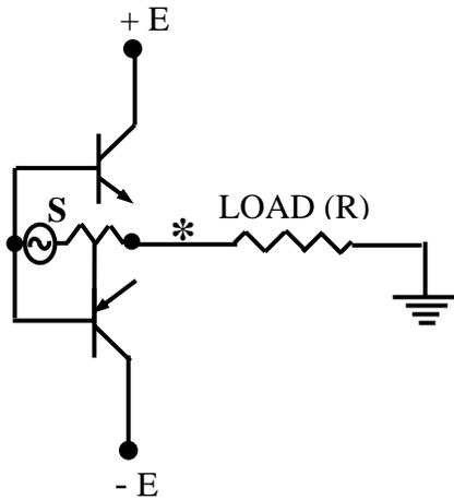
**Fig. 33.1 (a): A push-pull active amplifier circuit**
