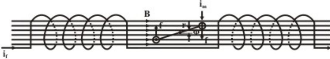
Fig. 43.1(b): Magnetic - field and torque developed in moving coil of an electro dynamoter.
