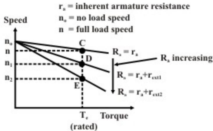
Figure 39.7: Family of speed vs. Torque current characteristic.
