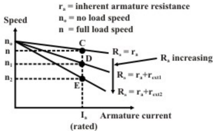
Figure 39.6: Family of speed vs. armature current characteristic.
