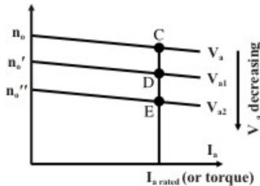
Figure 39.11: Family of  $n$  VS.  $I_a$  characteristics.
