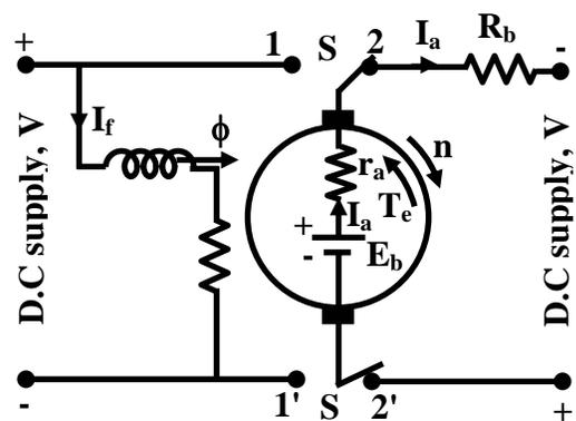
**Figure 39.26: Machine operates as generator during braking (plugging).**
