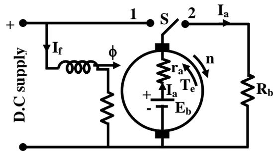
Figure 39.24: Machine operates as generator during braking
