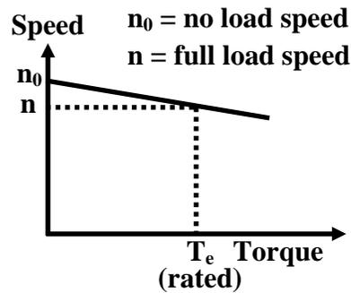
**Figure 39.5: Speed vs. torque characteristic.**
