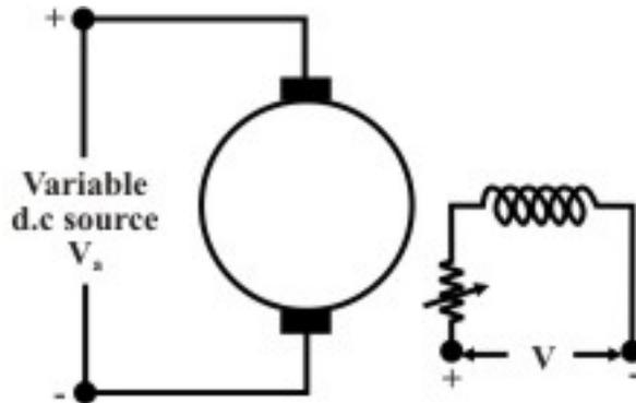
Figure 39.10: Speed control by controlling armature voltage.
