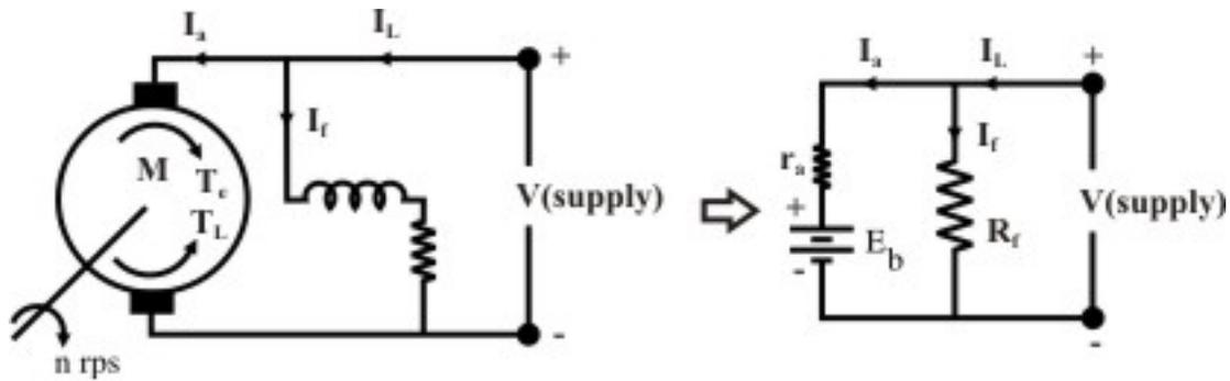
Figure 39.1: D.C shunt motor connection & its circuit representation.
