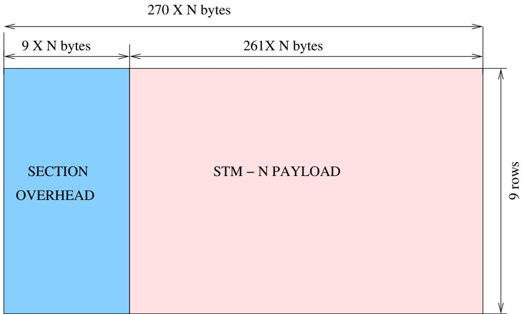
Out of the above  $9 \times 9 = 81$  bytes are section overheads while the remaining 2349 bytes form the payload. The higher rate frames are multiples of STM-1 and are labelled STM-N.
