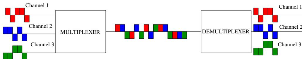
The way to achieve this is to divide the high rate channel into a series of time slots and the time slots could be assigned to the individual data stream.
