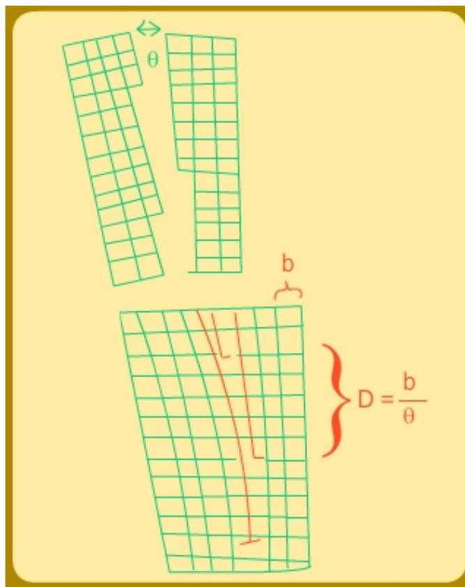
Figure 1: A wall of edge dislocations form a tilt grain boundary; it is a small angle grain boundary; the inter-dilocation separation in the grain boundary is decided by the misorientation between the two grains and the Burgers vector.
