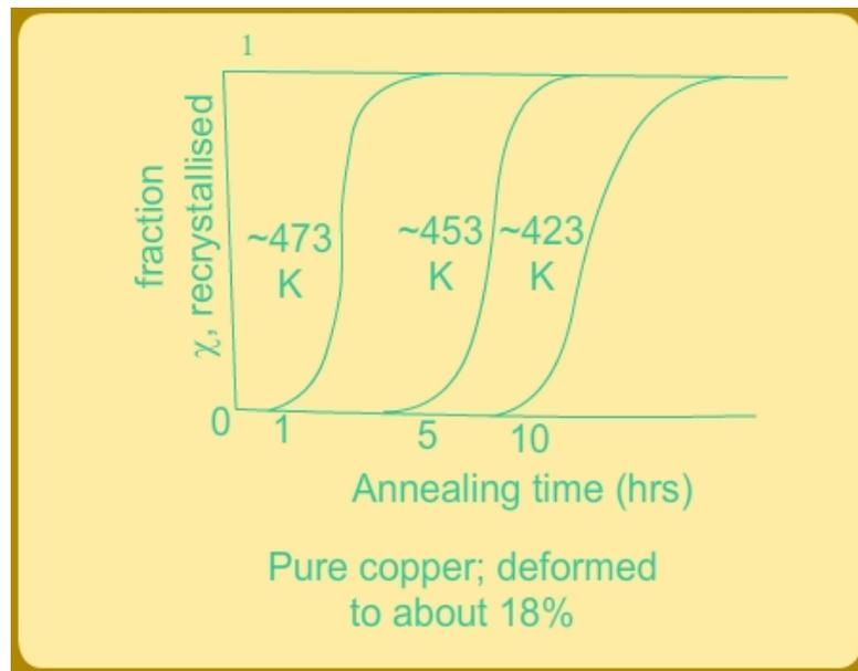
Figure 2: Annealing time versus fraction of recrystallised copper as a function of temperature. Note that the time changes from 1 to 5 to 10 hours with a decrease of about 20 K in temperature indicating the strong influence of temperature on recrystallisation kinetics.
