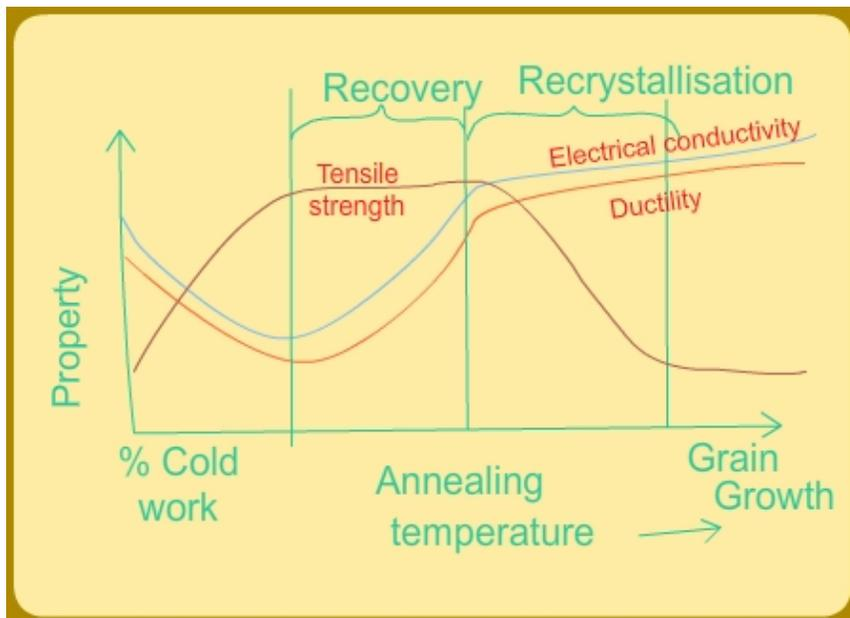
Figure 3: Changes in properties with % cold work and annealing temperature; increasing annealing temperatures leads to recovery and recrystallisation. Note that still higher annealing temperatures leads to grain growth.
