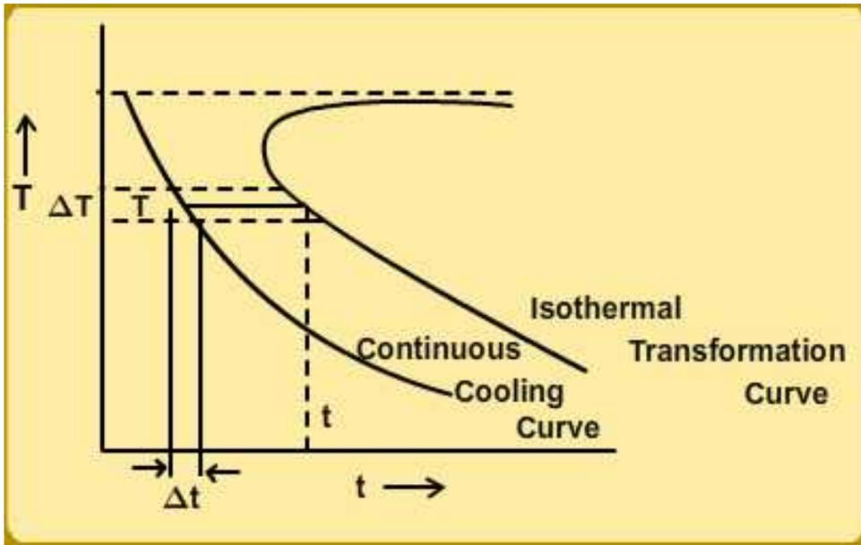
Figure 7: CCT and TTT diagrams.
