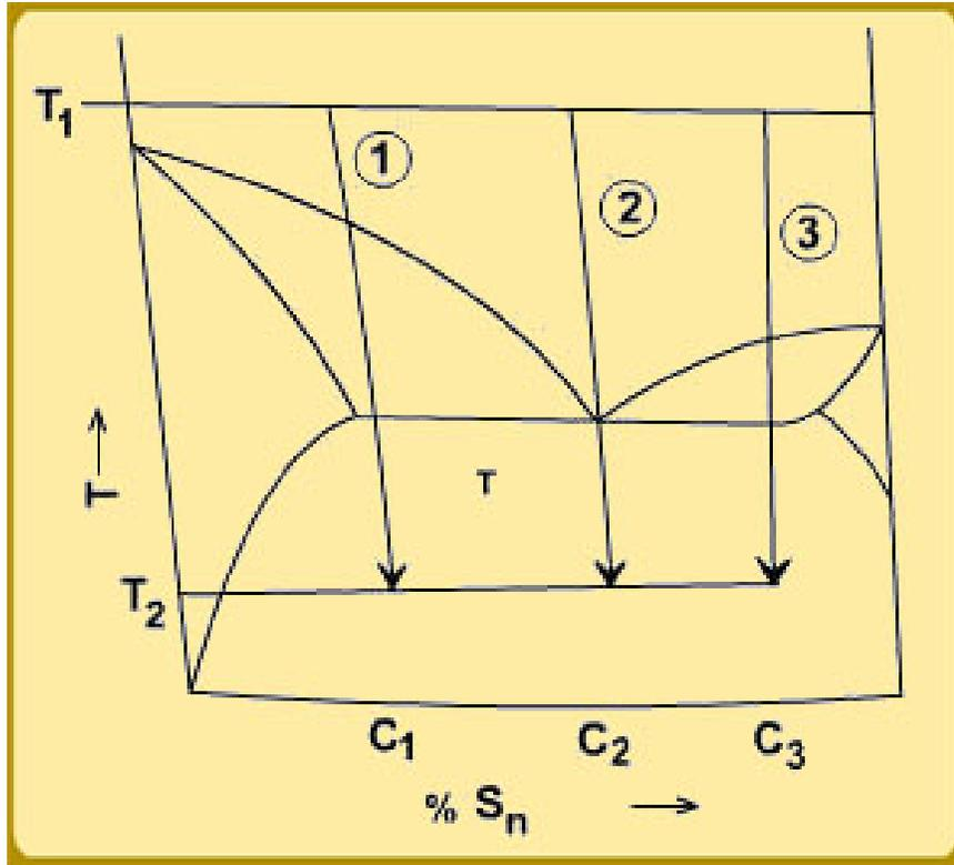
Figure 1: Pb-Sn phase diagram.
