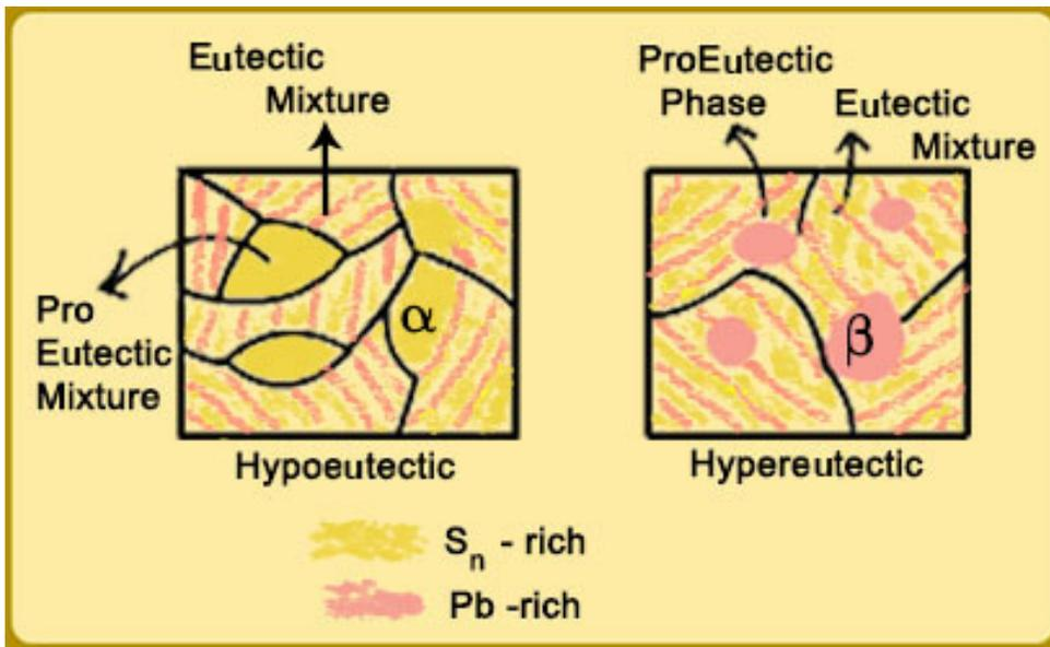
Figure 3: Hypo- and hyper-eutectic microstructures.
