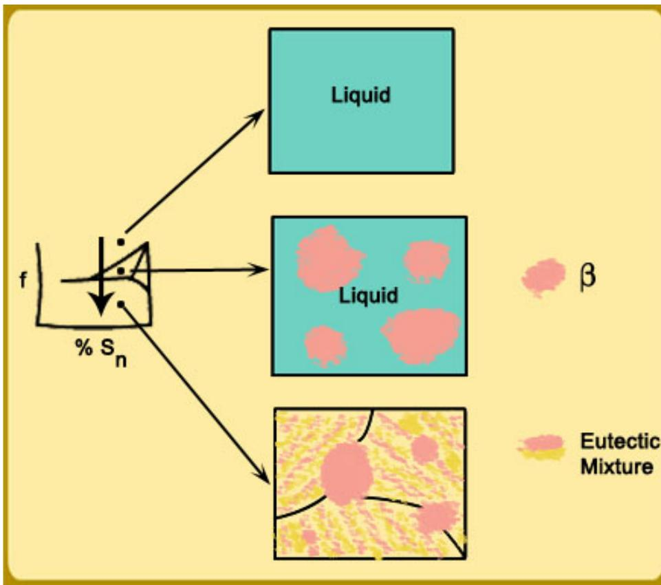
Figure 4: Formation of microstructure in an off-eutectic alloy.
