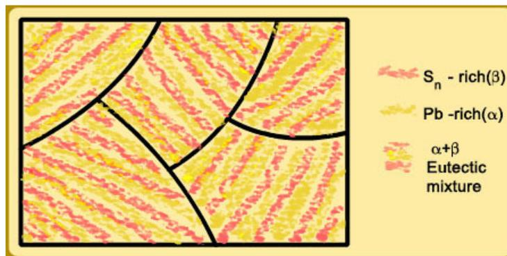
Figure 2: Eutectic microstructure.
