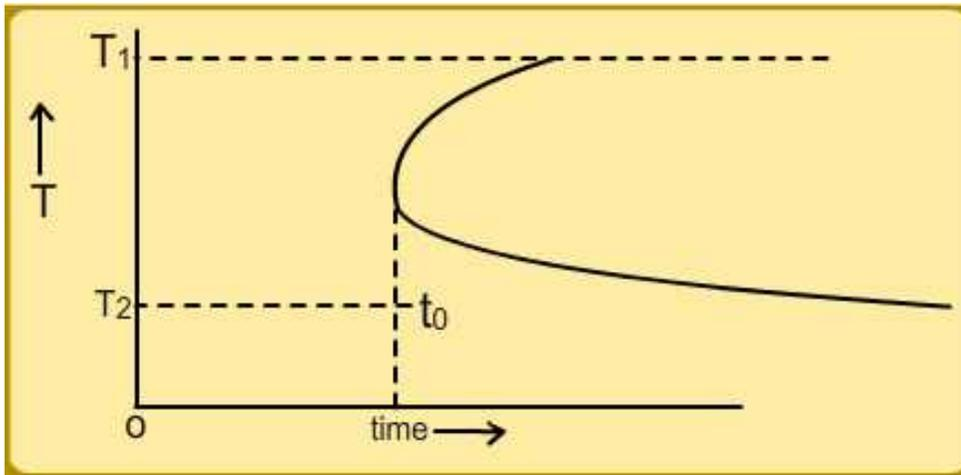
Figure 5: Fast quench for the suppression of second phase formation.
