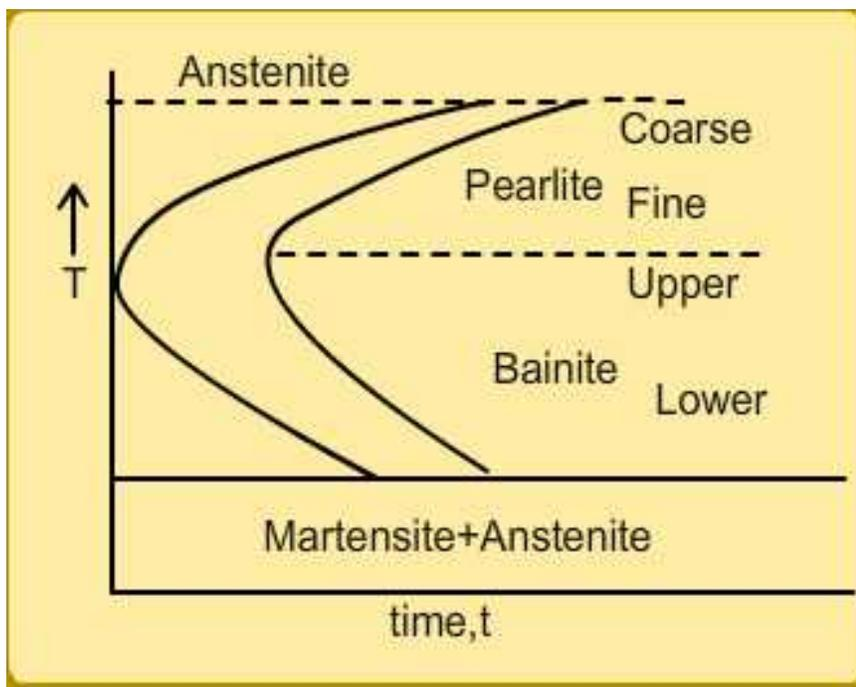
Figure 6: Schematic TTT diagram in eutectoid steel.
