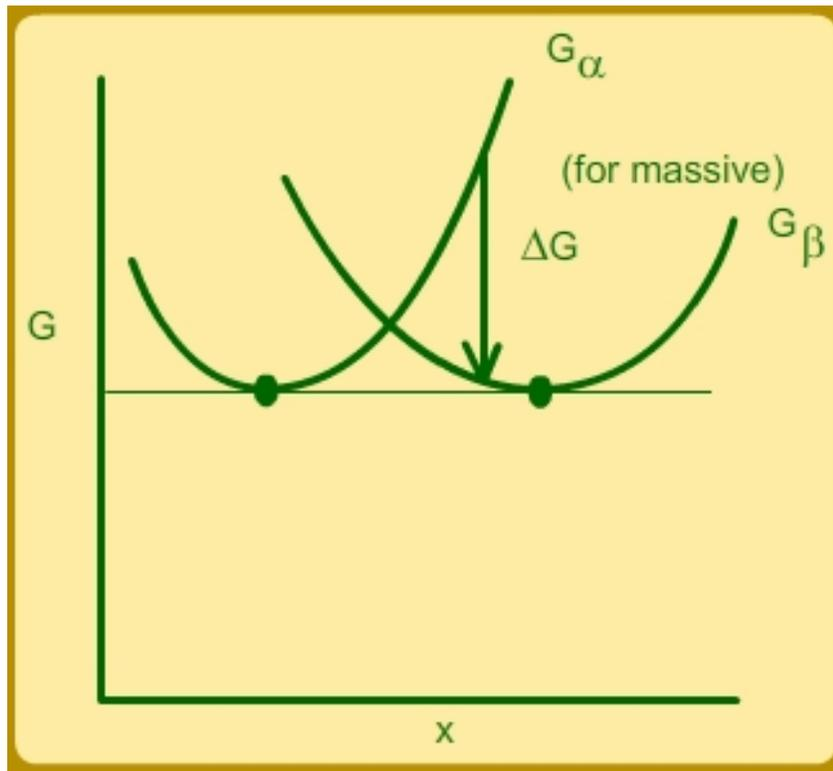
Figure 35: Driving force for massive transformation.
