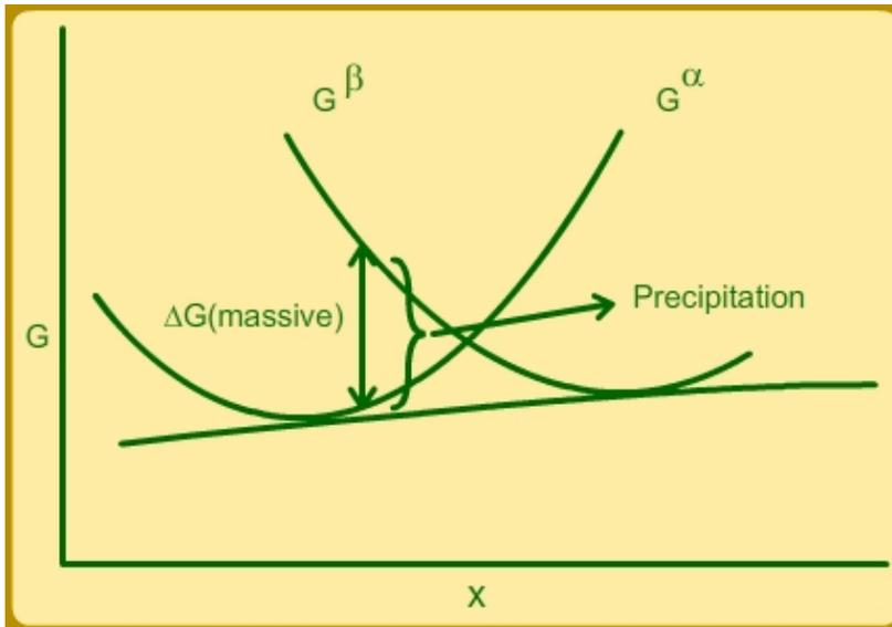
Figure 37: Massive transformation in a two phase region.
