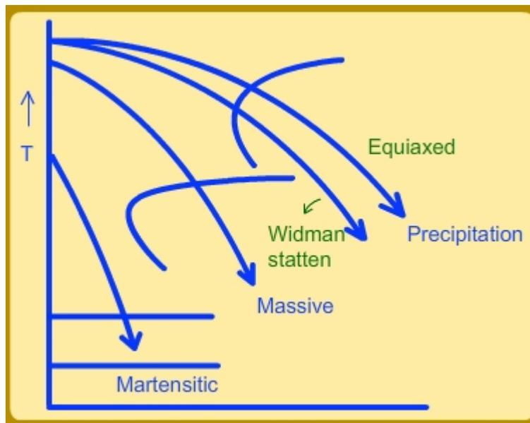
Figure 34: CCT diagram showing precipitation, Widmanstatten growth, massive transformation and martensitic transformations.
