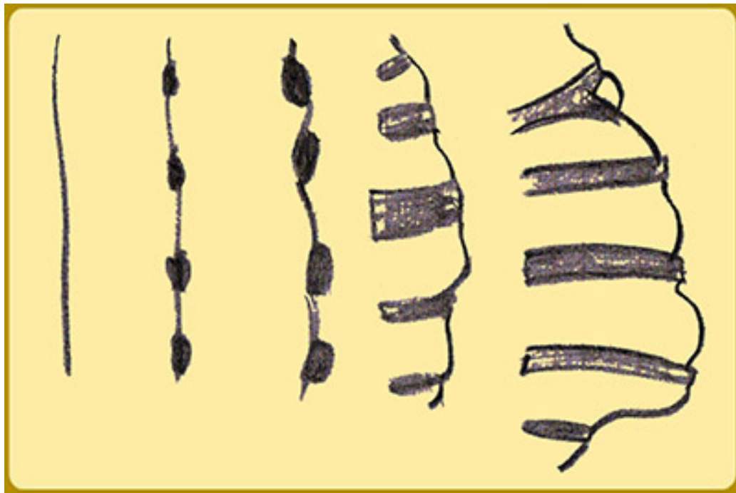
Figure 19: Mechanism of formation of cellular precipitates.
