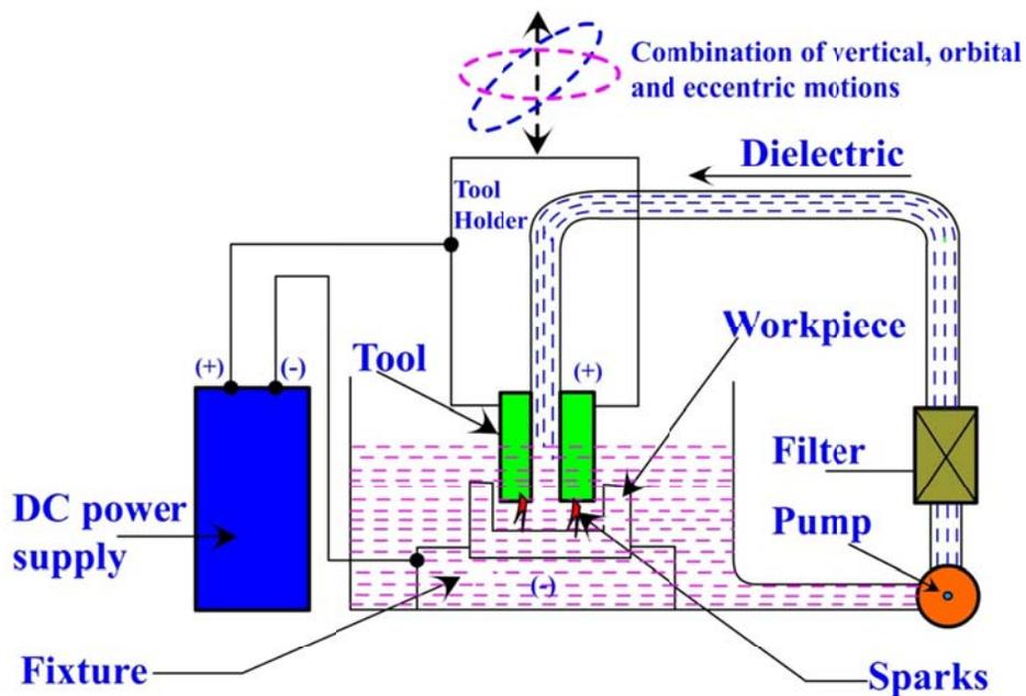
**Fig. 3.9.1 Schematic of Electric Discharge Machining**
