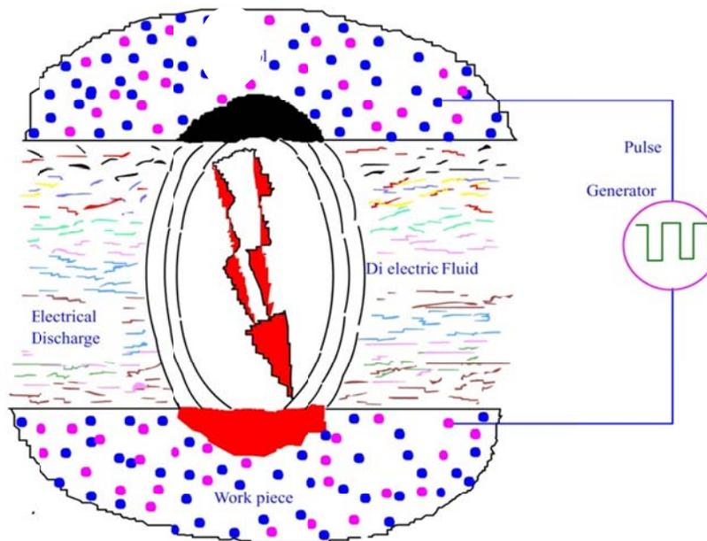
**Figure 3.9.2 Close View of ED Machining region**
