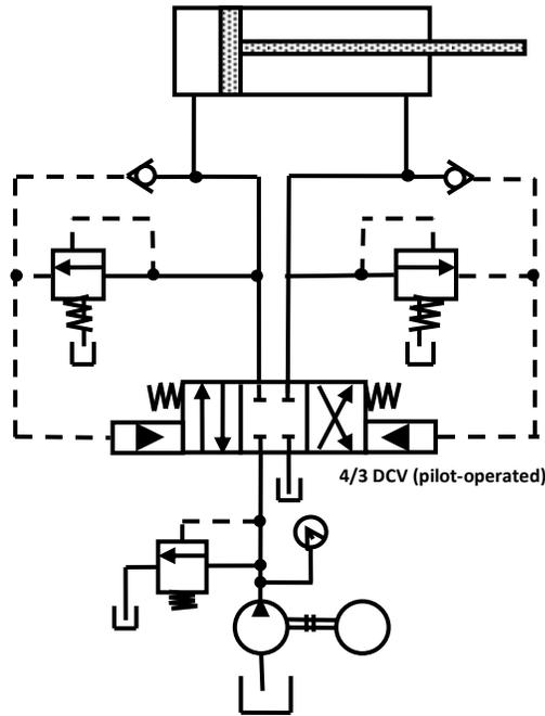
**Figure 1.8** Sequencing circuit.
