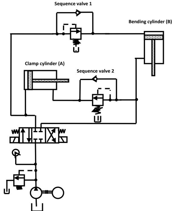
**Figure 1.7** Sequencing circuit.
