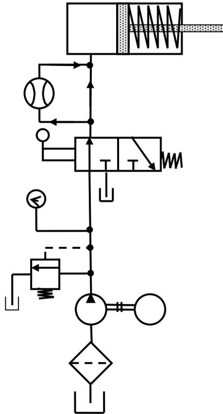
**Figure 1.1** Control of a single-acting cylinder.
