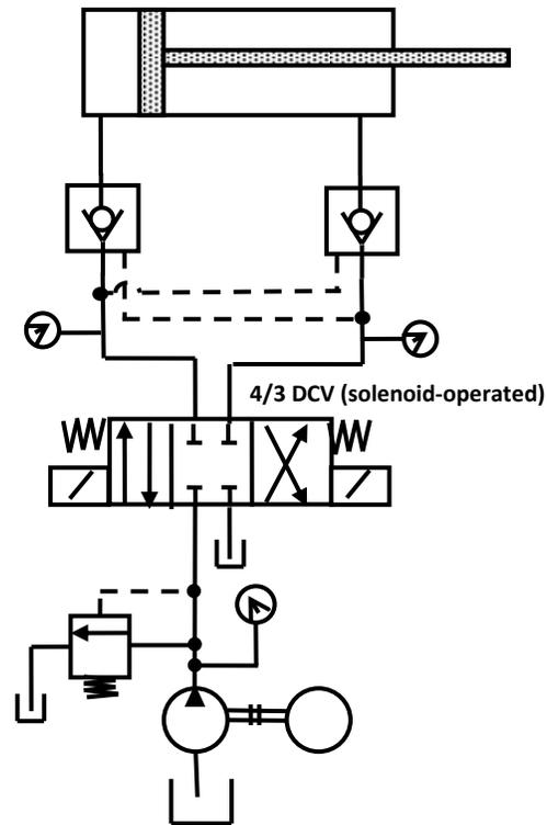
**Figure 1.9** Locked cylinders with pilot check valves.
