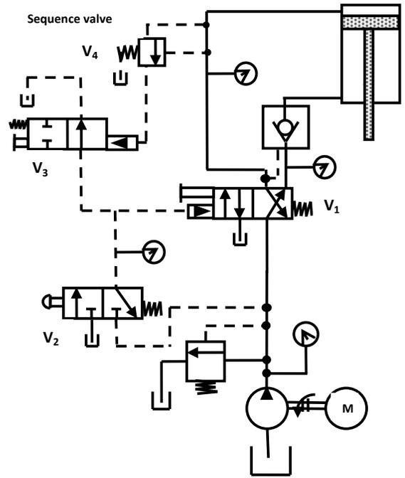
**Figure 1.14** Fail-safe circuits –overload protection.
