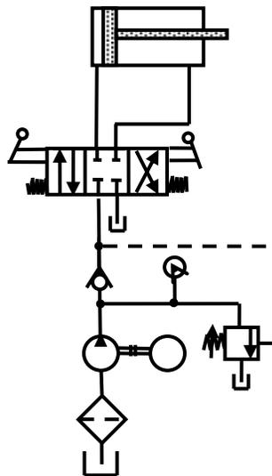
**Figure 1.4** Pump-unloading circuit.
