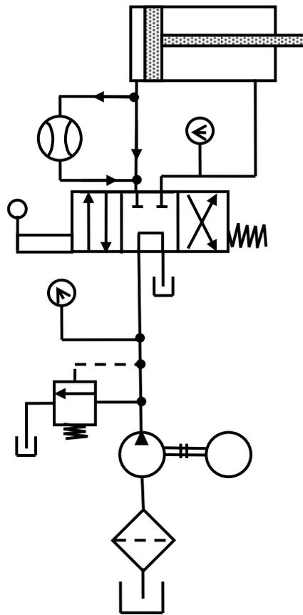
**Figure 1.2** Control of a double-acting cylinder.
