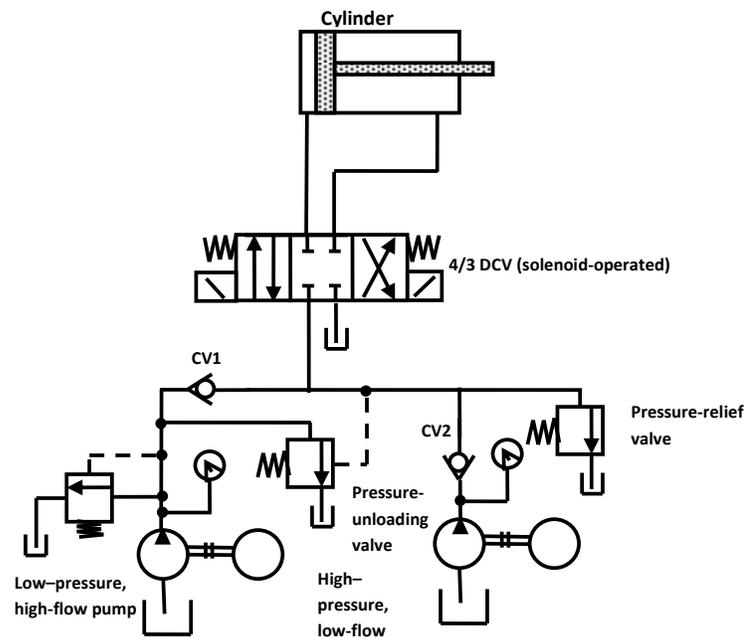
**Figure 1.5** Double-pump circuit.
