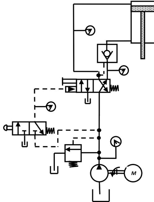
**Figure 1.13** Fail-safe circuits – inadvertent cylinder extension.
