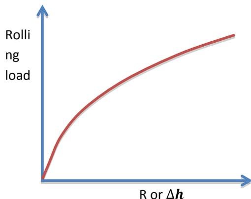
**Fig. 1.1.1: Variation of rolling load with roll dia or strip thickness reduction**
