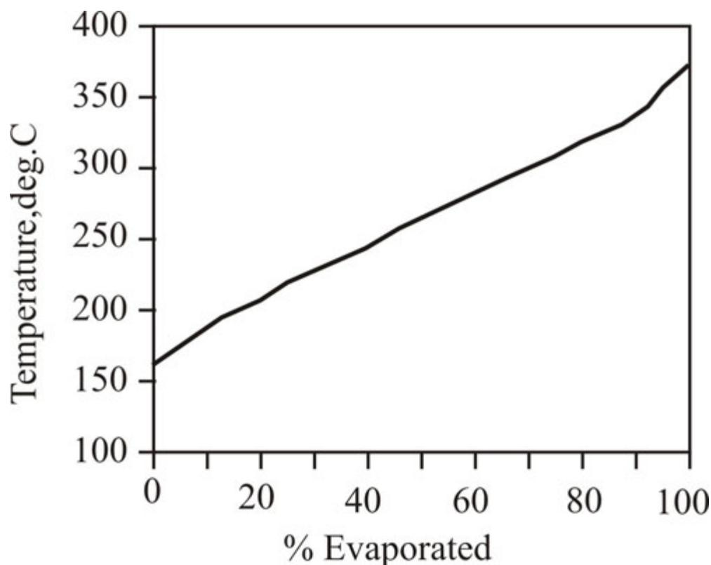
Figure 8.6 Typical distillation characteristics of diesel fuel.
