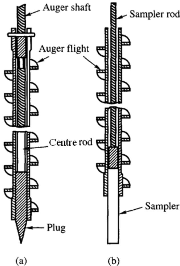
**Figure 1.2 Hollow-stem auger**
