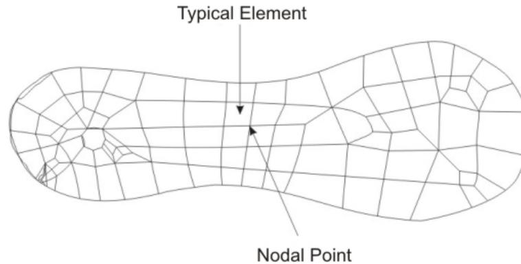
**Fig. 1.1.3 Finite element discretization of a domain**
