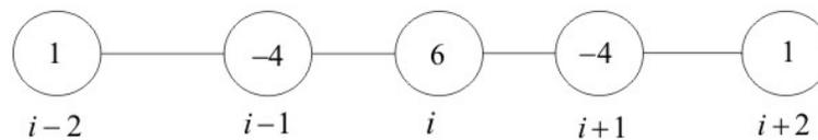
**Fig. 1.1.2 Finite difference equation at node i**
