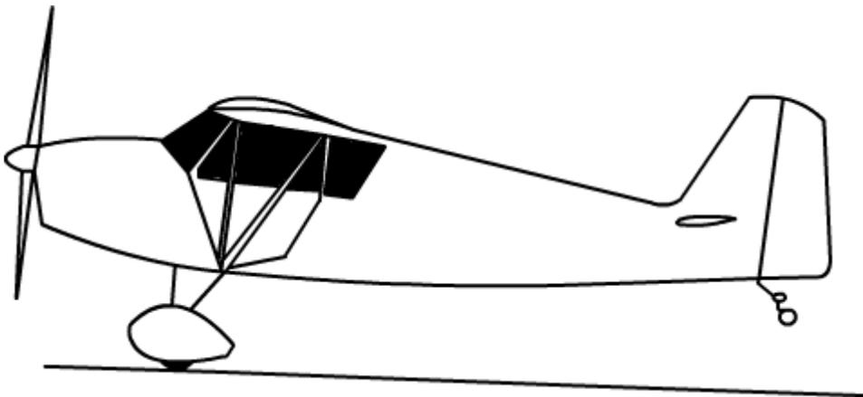
Fig.10.1d Tail wheel type of airplane during middle part of take-off run
