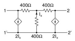
Determine the y-parameters of the circuit above.
