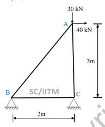
2. Using stiffness method of analysis, find the reactions of the truss shown in figure below:
