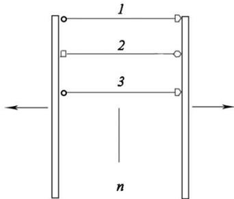
The system function for a parallel system is
