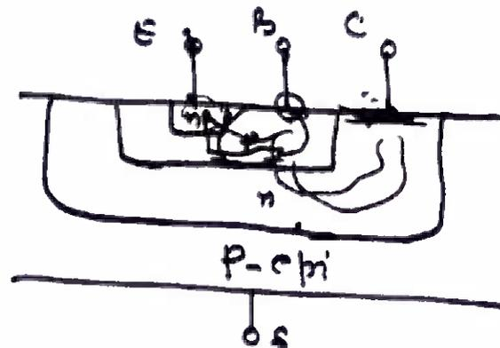
Since in an IC, collector is a diffused region in substrate, one observes presence of a collector-substrate junction with capacitance
