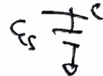
Normally substrate is grounded. Hence  $C_{cs}$  is the collector capacitance between collector terminal & ground
