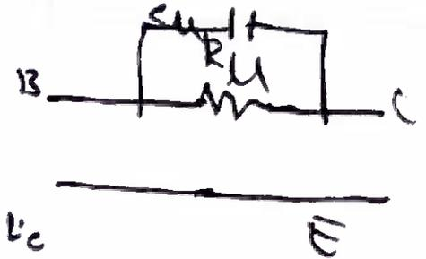
Collector Substrate Capacitance  $C_{cs}$
