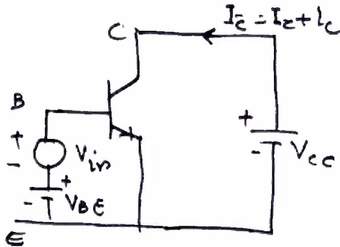
$$I_e = I_s \exp\left[\frac{V_{BE} + V_{in}}{V_T}\right] \quad \text{Total}$$
