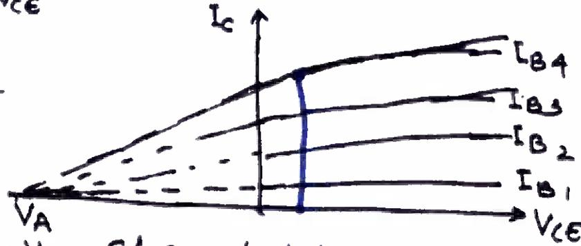
$\therefore$  Output Resistance  $r_o = \frac{\Delta V_{CE}}{\Delta I_c} = \frac{V_{CE}}{i_c} = \frac{V_A}{I_c}$
