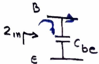
At lower frequency  $Z_{in} = \frac{1}{j\omega C_{be}}$  is large
