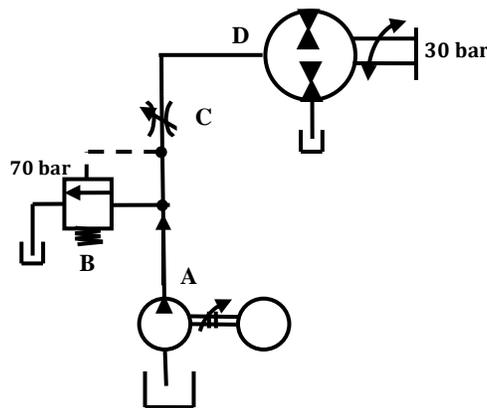
Figure 2 : Speed control of hydraulic motor
