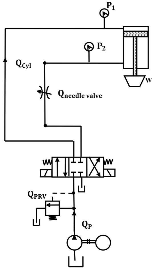
**Figure 3 : Hydraulic cylinder with suspended weight**
