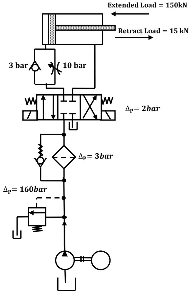
**Figure E4 : Hydraulic cylinder with meter in control**
