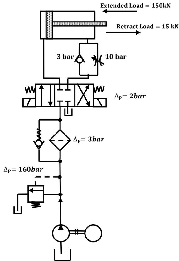
**Figure E5 : Hydraulic cylinder with meter out control**
