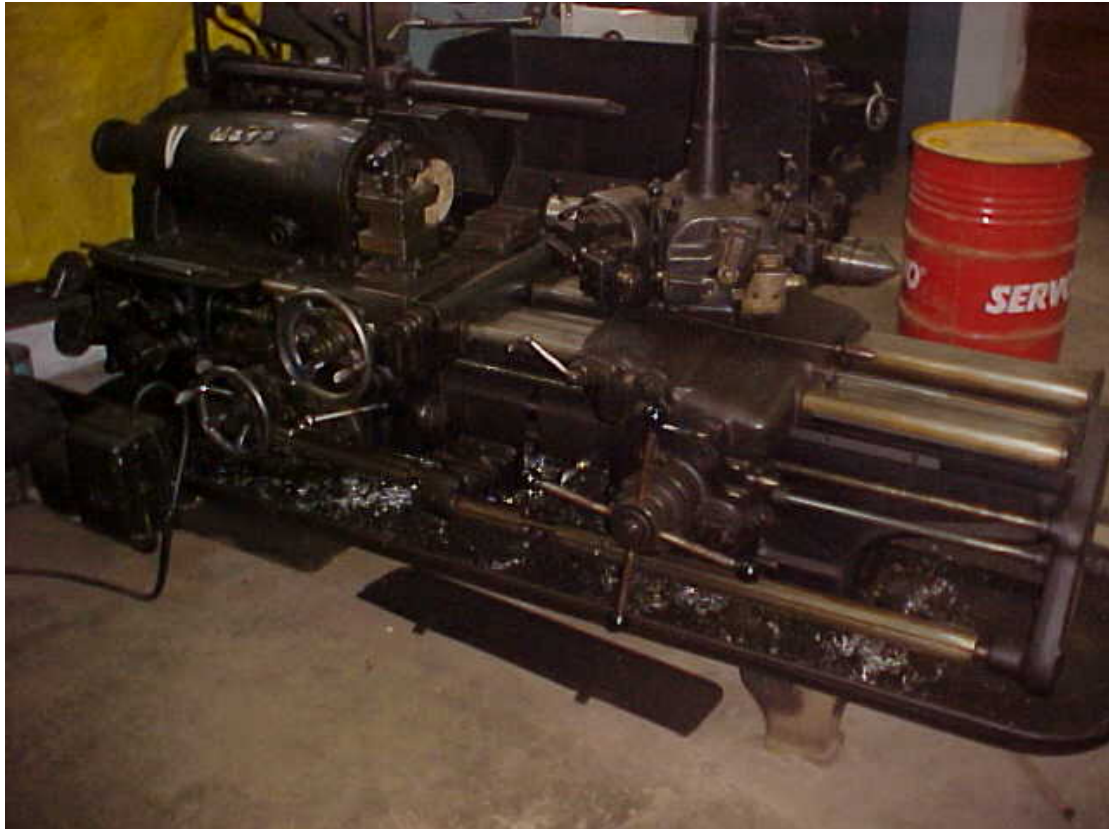
Fig. 4.7.4 Pictorial view of a turret lathe.
