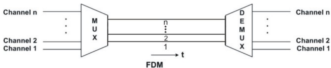
Figure 2.7.2 Basic concept of FDM
