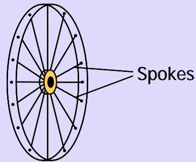
**Figure 1-1.2** Pre-tensioning the spokes in a bicycle wheel
