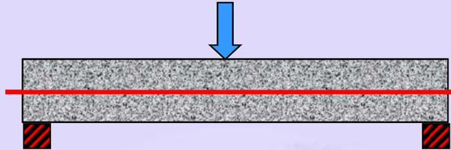
**Figure 1-1.4** A prestressed beam under an external load
