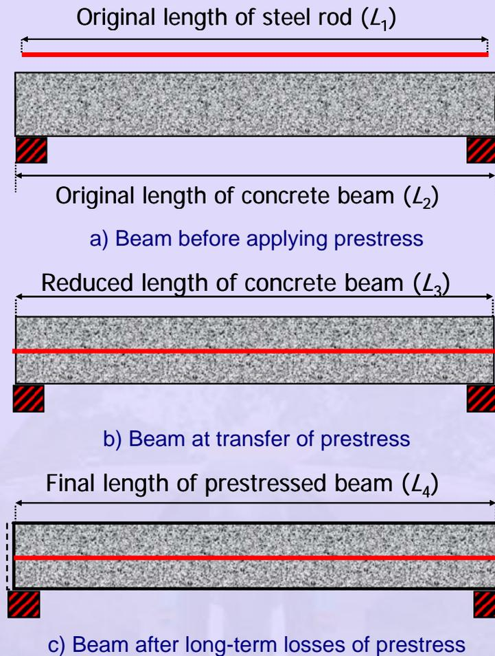
**Figure 1-1.5** Variation of length in a prestressed beam
