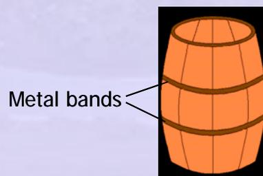
**Figure 1-1.1** Force-fitting of metal bands on wooden barrels
