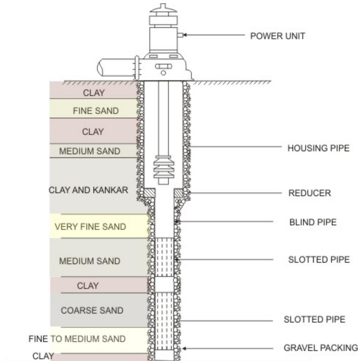
FIGURE . 11 TYPICAL INSTALLATION OF TUBE WELI
