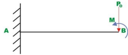
Fig.23.2(a) Cantilever beam
