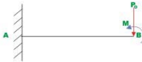
Fig.23.3(a) Cantilever beam
