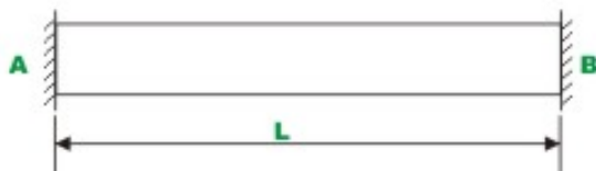
Fig. 9.4 Fixed - fixed beam
