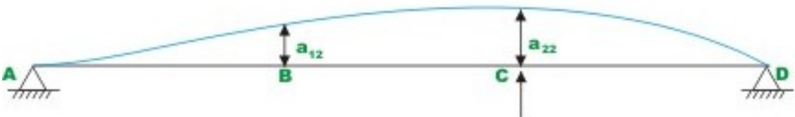
Fig. 9. 7 (d) Primary structure with unit load along R 2
