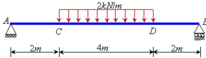
**Figure 6.6 Uniformly distributed load acting on a beam**
