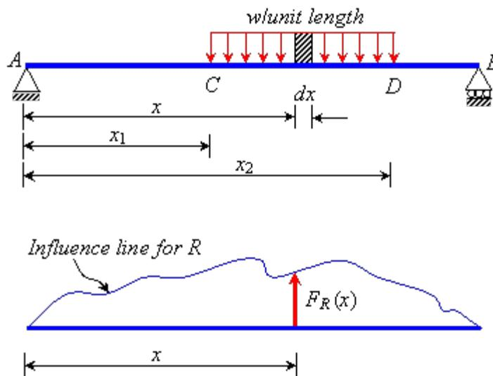
Figure 6.5 Using influence line for a uniformly distributed loading
