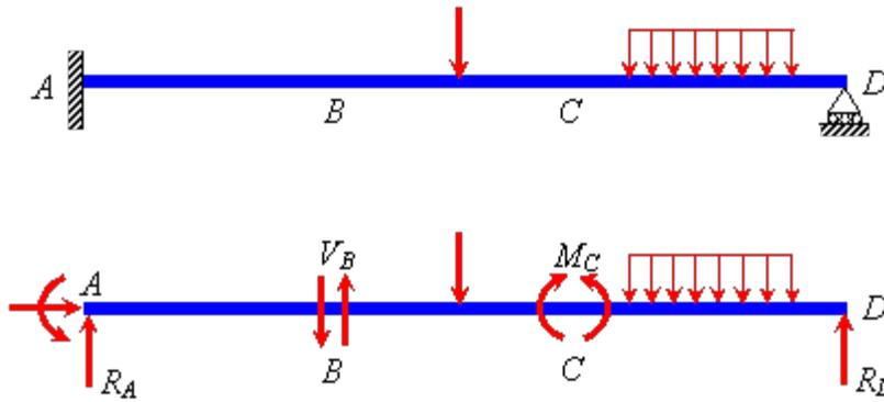
Figure 6.2 Different response parameters for beam  $AD$
