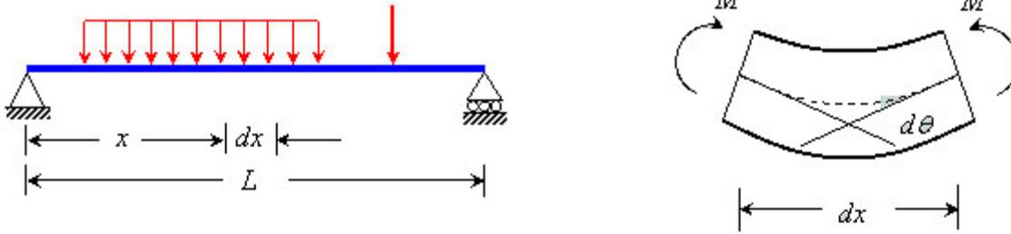
Figure 4.25 Member under bending
