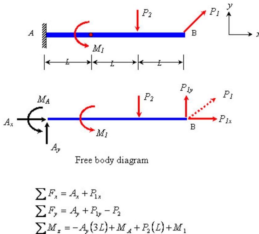
Figure 1.8 Obtaining resultants for a cantilever system
