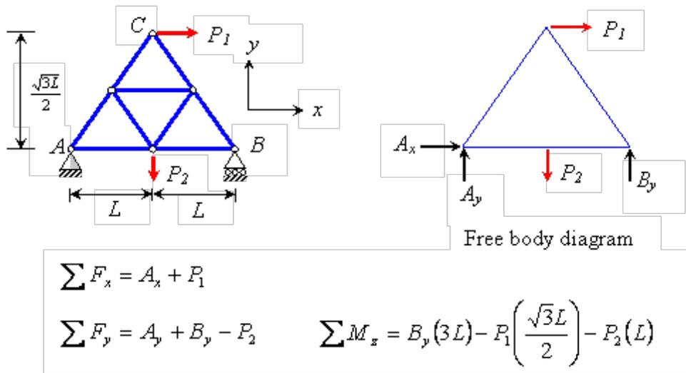
Figure. 1.7 Obtaining resultants for a truss
