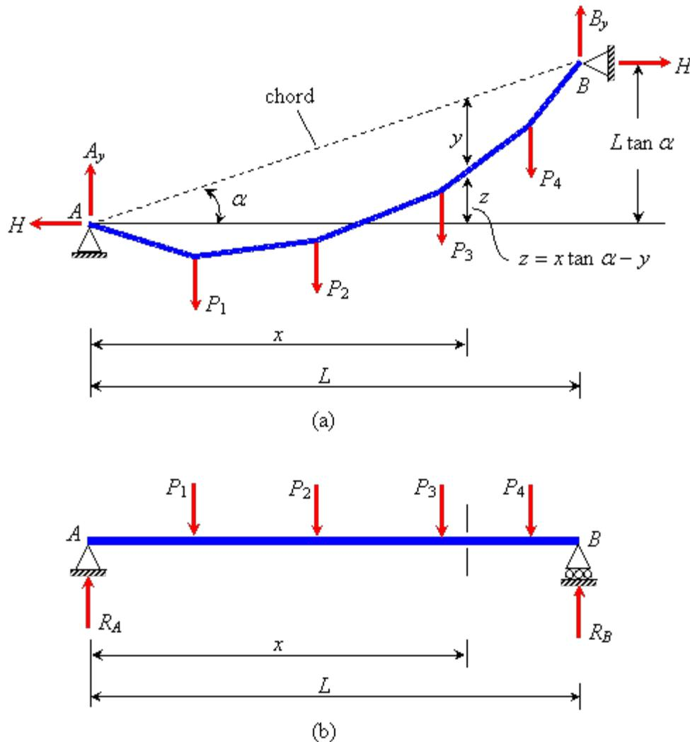
**Figure 3.4 Explanation of the general cable theorem: (a) Cable under vertical loads, and (b) Simply supported beam with equal span under the same set of loads**
