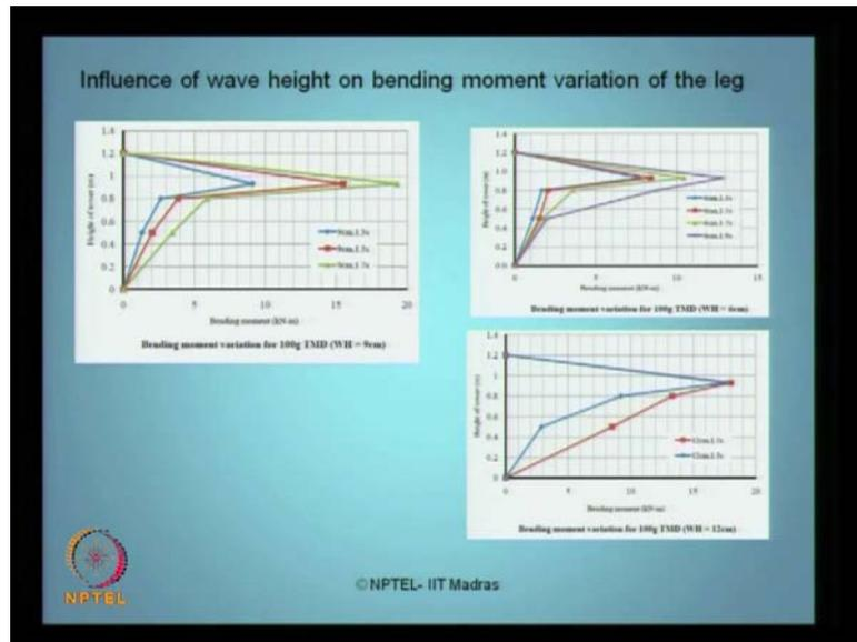
Let us see what happens when I change the wave heights, because the earlier case were constant wave height. Now, I change the wave height for TMD 100 grams, 9 centimeter, 6 centimeter, 12 centimeter, I am changing the wave height, of course the plot is also showing different period as well. Again you see qualitatively the bending moment maximum occurs for all the cases at the same point, right? But there is a reduction quantitatively in the bending stress or in the bending moment.
