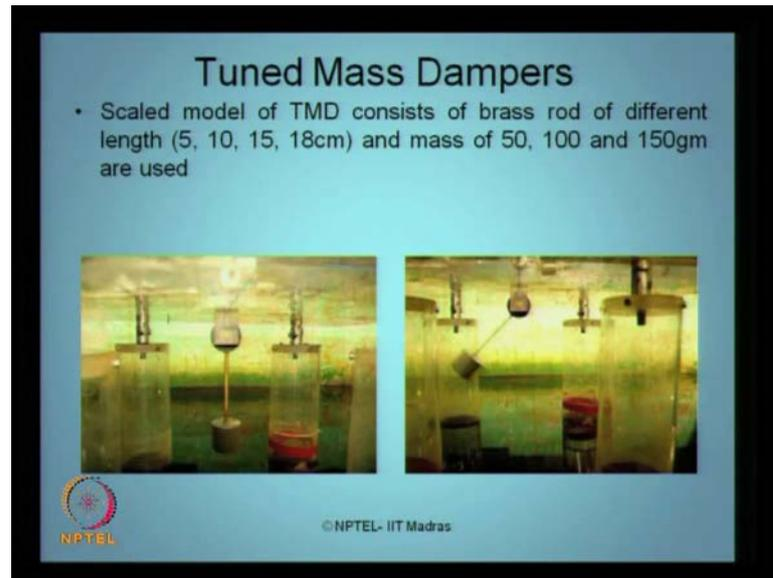
The scale model of T M D of brass rod of different lengths of different 5, 10, 15, 18 centimeter have been tested with different mass of 50, 10, 100, 150 and 230 I have been used in the study, which corresponds to the mu ratios of various percentage as we analyzed in the previous example.
