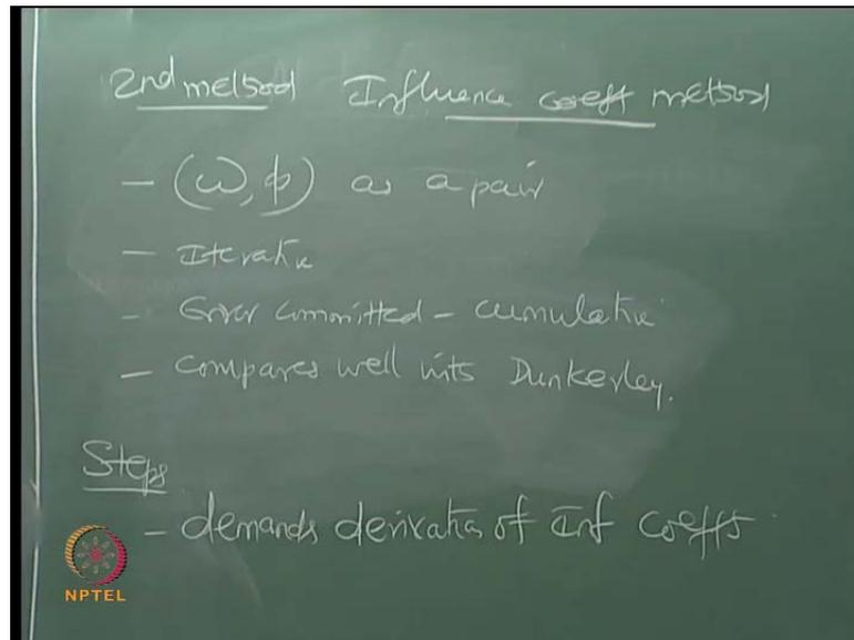
So, the second method is called influence coefficient method. This method will give me omega and phi as a pair. This method is iterative and the error committed would be cumulative and this method compares well with Dunkerley. Let us see what this method is. This method also demands steps, this method also demands derivation of influence coefficient. So, let us derive the influence coefficient first for the next example, which I show here.
