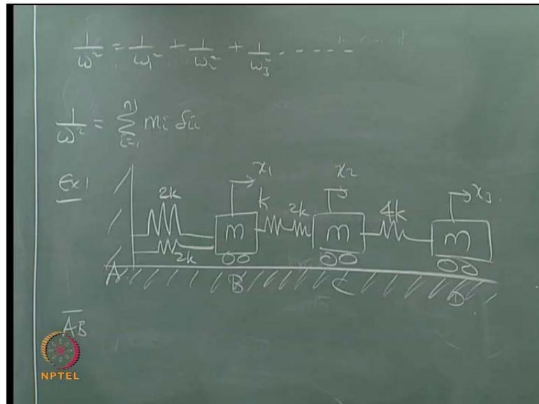
So, if you want to find a 3-D model, for example, let us say,  $1/\omega^2$  should be  $1/\omega_1^2 + 1/\omega_2^2 + 1/\omega_3^2$  and so on. It is an approximation made by Dunkerley, which can be applied to multi-degree and he says simply,  $\sum m_i \delta_{ii}$  will give me  $\omega^2$ . So, we will take up simple example and see how this can be demonstrated, we will take up an example.
