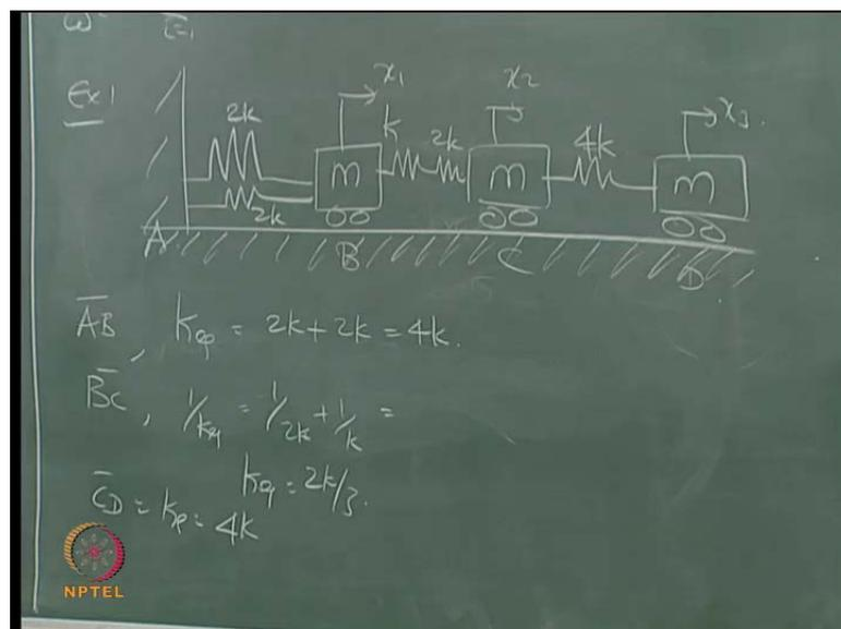
So, degree of freedom one, degree of freedom 2... So, let me name these segments as A, B, C and D for segment AB. I can work out equivalent stiffness. So,  $k$  equivalent is  $2k$
