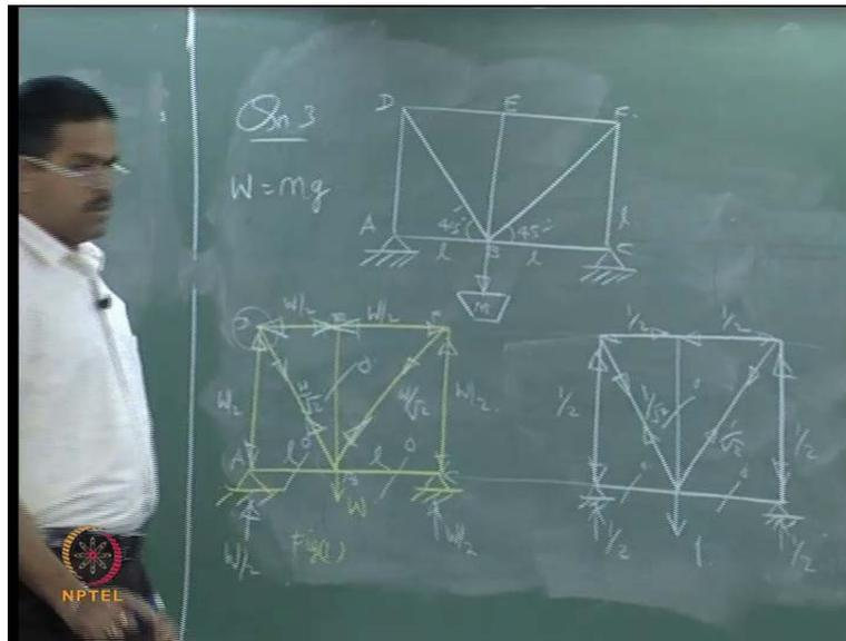
Question number three, direct application problem, let us say, I have an offshore platform whose deck is supported by a truss system; whose deck is supported by a truss system. A typical truss system is shown, I am drawing it here though in reality, the truss system for which an offshore platform deck is supported will be complex, but I am taking a very simple system for demonstration.
