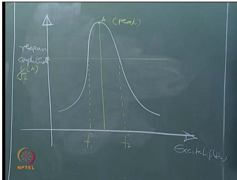
Now, I try to plot at  $\beta = 1$ , I vary only the excitation frequency because I know  $\omega_n$  value. So, for different excitation frequency in Hertz I try to plot the response amplitude. Let us say the plot, what I get from this by varying  $\omega$  alone for a specific  $\omega_n$  appears like this. So, obviously, there will be a peak, which you will get when these values are equal, I call this peak as A, which is the peak of this response.
