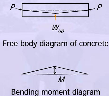
**Figure 3-2.6** Simply supported beam with singly harped tendon
