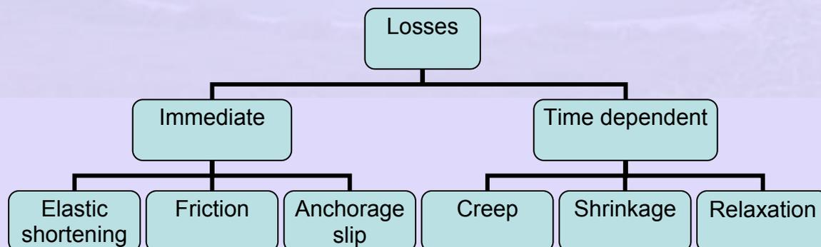
**Figure 2-1.3** Causes of the various losses in prestress
