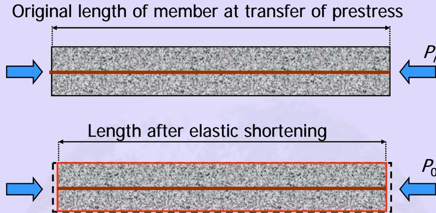
**Figure 2-1.4** Elastic shortening of a pre-tensioned axial member
