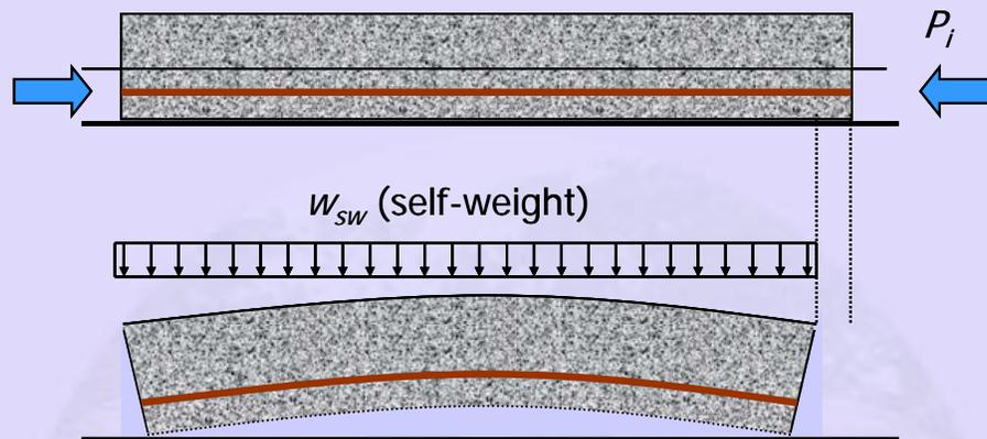
**Figure 2-1.6** Elastic shortening of a pre-tensioned bending member
