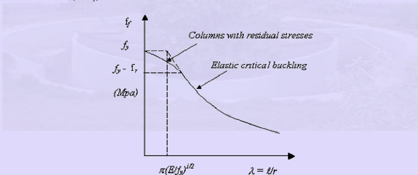
**Fig 5.13 Strength curve for columns having residual stress**
