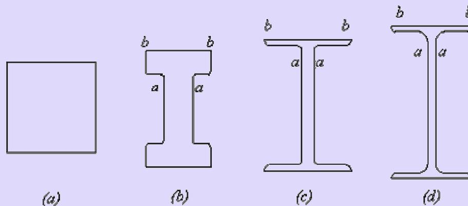
**Fig 5.11 Various stages of rolling a steel girder**
