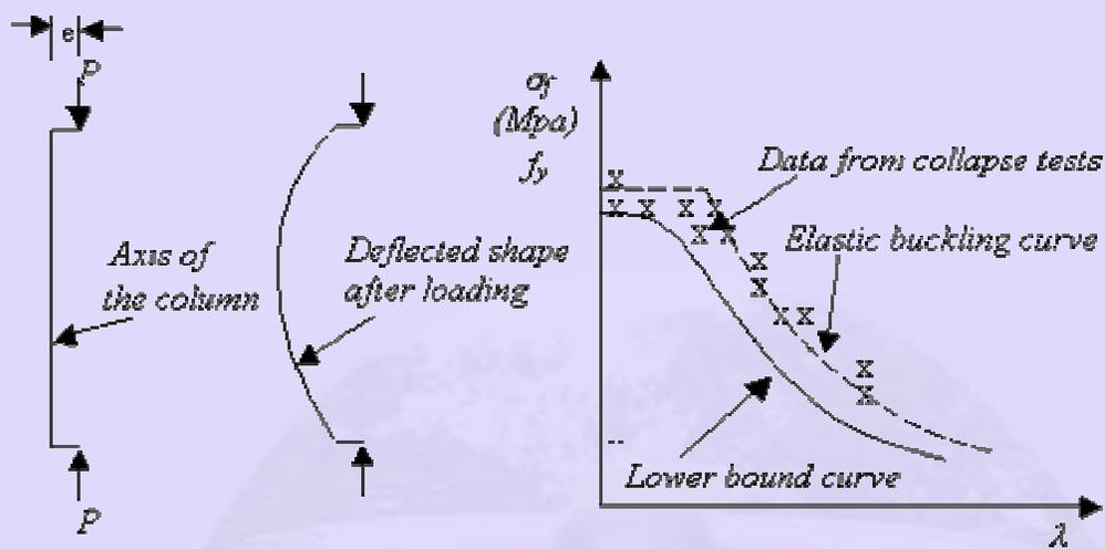
**Fig 5.10 Strength curves for eccentrically loaded columns**
