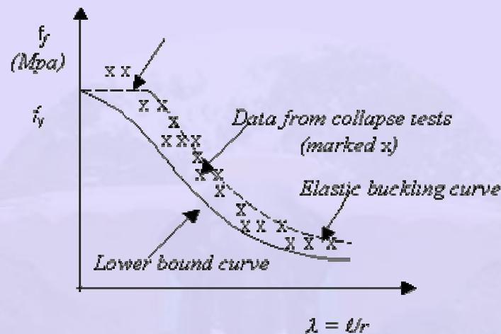
**Fig 5.9 Strength curves for strut with initial imperfection**
