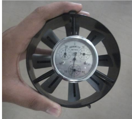
Fig. 2 Right way to hold vane anemometer during traversing
