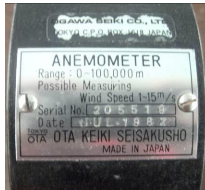
Fig. 5 Manufacturer's name and other details printed on anemometer
