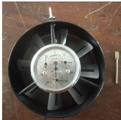
Fig. 3 Vane anemometer with reset pin at its right
