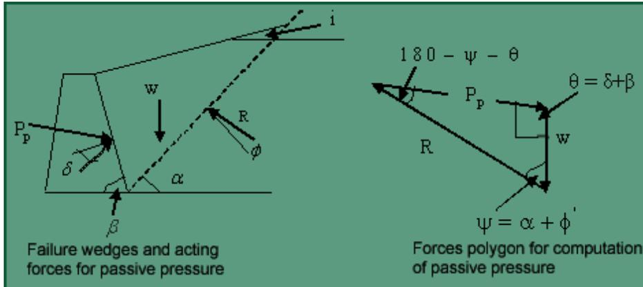
**Fig. 2.14 Failure wedges**
