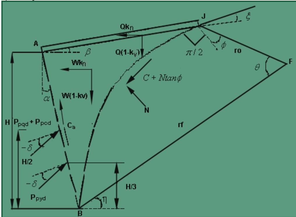
Fig. 2.24 Logarithmic Failure Surface and the Forces Considered
