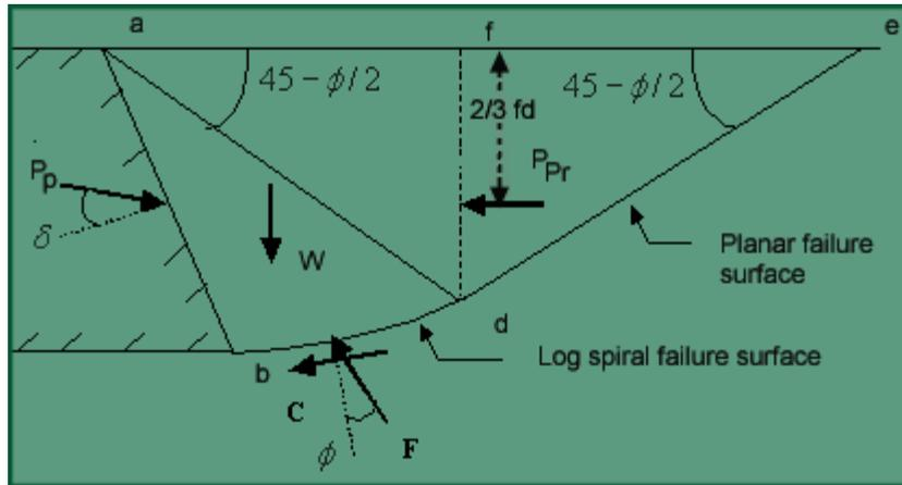
Fig. 2.19 Rupture Surface assumed in Terzaghi's Wedge Theory
