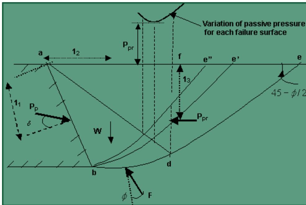
Fig. 2.20 Logarithmic Spiral Method for Determining Passive Earth Pressure
