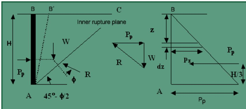
**Fig. 2.10 Rankine's passive earth pressure in cohesionless soil**
