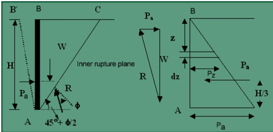
Fig. 2.9 Rankine's active earth pressure in cohesionless soil
