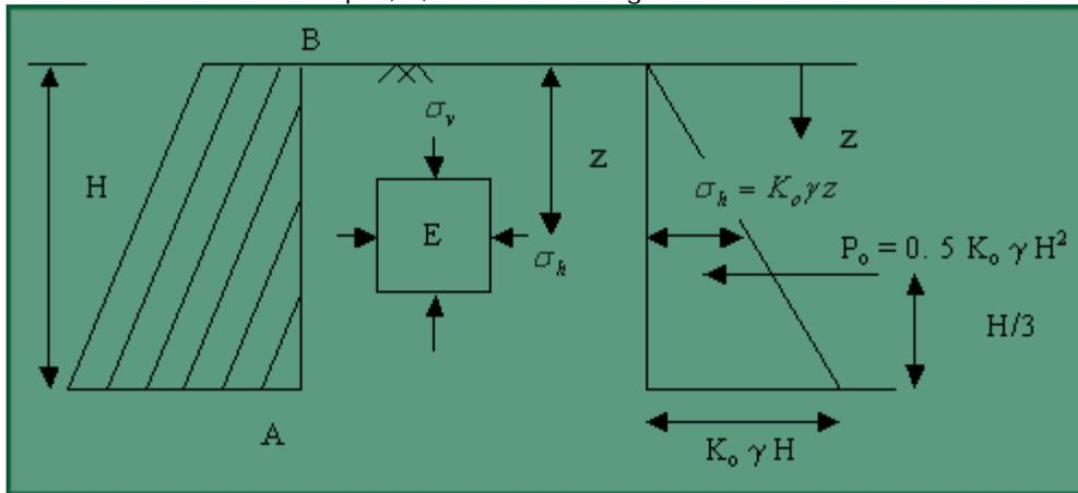
Fig. 2.8 Lateral earth pressure for at rest condition.
