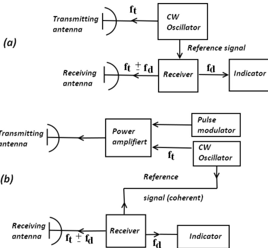
Figure 4.1: Block Diagram of (a) Simple CW Radar and (b) pulse radar using doppler information
