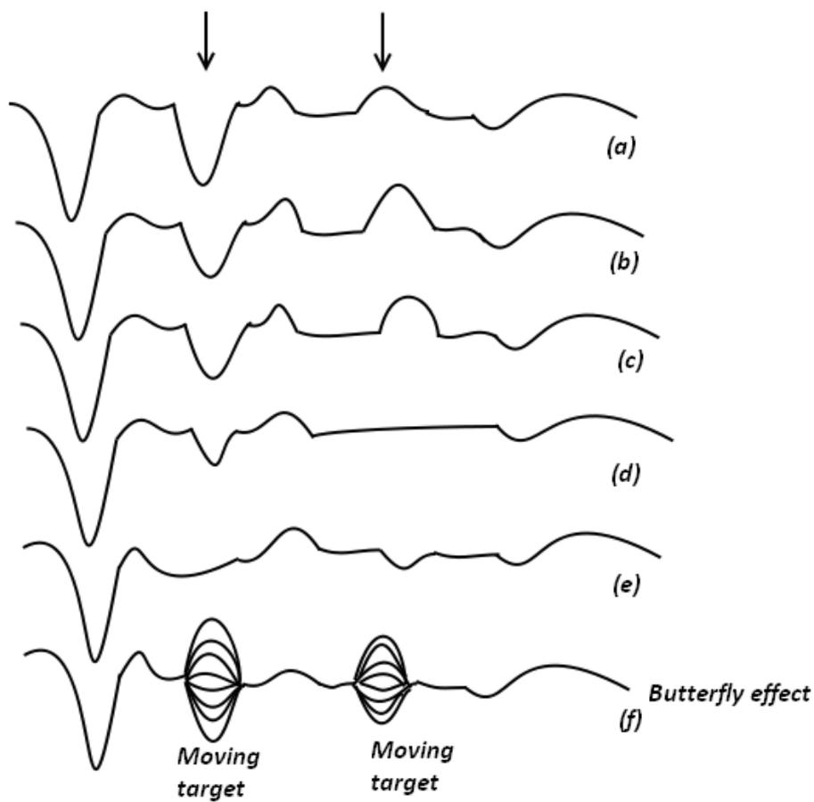
Figure 4.4: (a-e) Successive sweeps of an MTI Radar on an A-scope display and (f) supersposition of these signals (arrows indicate moving targets)
