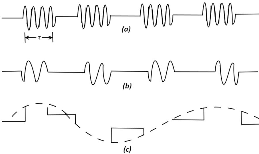
Figure 4.3: (a) Reflected signal (b) Difference signal when  $f_d > 1/\tau$  (c) Difference signal when  $f_d < 1/\tau$
